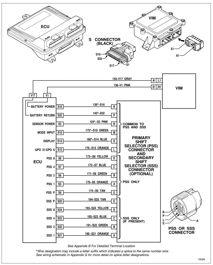
Figure 5–4. Code 23 Schematic Drawing
