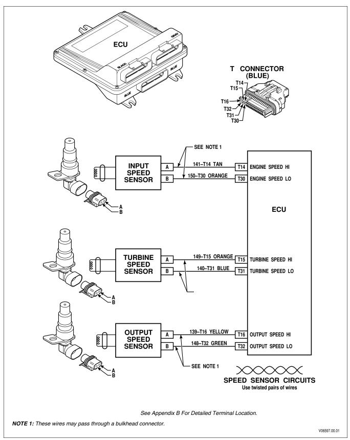
Figure 5–3. Code 22 Schematic Drawing
