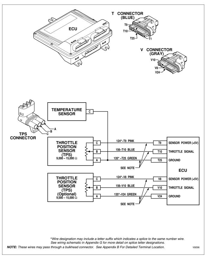
Figure 5–2. Code 21 Schematic Drawing
