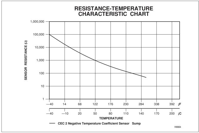
Figure 5–6. Temperature Sensor Chart
