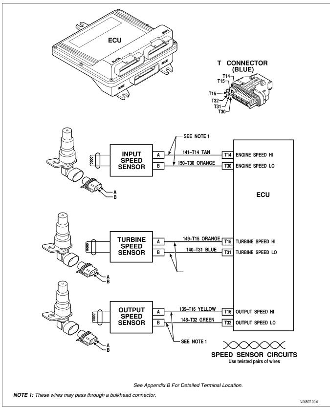
Figure 5–7. Code 25 Schematic Drawing
