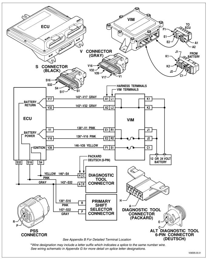
Figure 5–1. Code 13 Schematic Drawing
