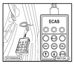
■ Operated by remote control device, placed in the holder on the rear wall of the cab, in extended cab versions at the driver's seat.
