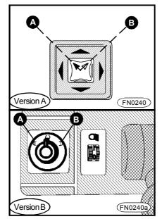
■ Turn the controller to select adjustment of the left or right mirror.
