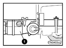
■ The tank "usable capacity" (item 1) is 23 I (total capacity 30 I).
