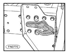
There is a special hook welded to the left bracket on the rear bumper to hold a rope in case of recovery.
