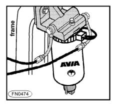
Unscrew drain bolts on the fuel filter bottom to allow draining of water from the fuel filter. When all dirt particles drip out, screw the bolts again.
