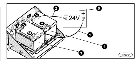
■ The vehicle with a discharged battery may be started only by connecting it to the battery of some other vehicle with the same nominal voltage.
