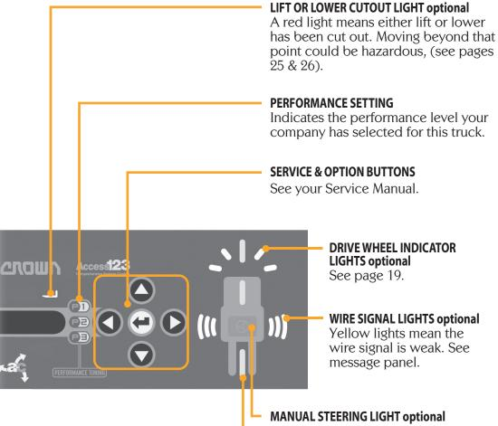
A red light means you are in manual steering mode. Take control of the steering tiller.
