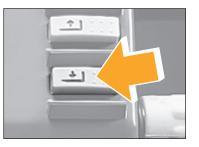
Push the Lower button to lower the platform and forks. Release the button when you reach the desired height.
