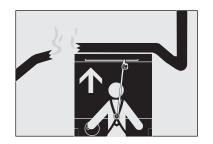
To travel past the cutout height, push the Override Switch while, at the same time, pushing either the Raise or Lower button.
