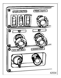
Figure 9 Typical Cruise Control Switches
