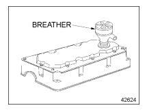
Figure 20 Rocker Cover-Mounted Breather
