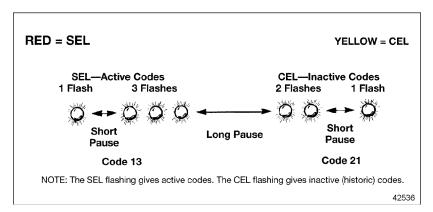
Figure 8 SEL/CEL Flashing Code Examples
