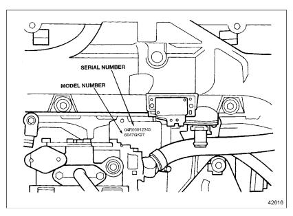
Figure 1 Location of Engine Serial and Model Numbers
