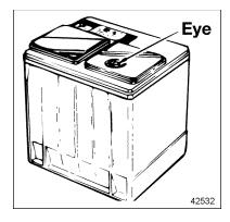
Figure 5 Check "Eye" of Maintenance-Free Batteries
