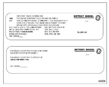
Figure 3 Typical Engine Certification Labels
