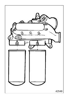
Figure 23 Spin-On Oil Filters
