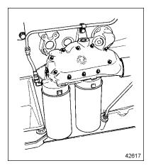
Figure 16 Lubricating Oil Filters
