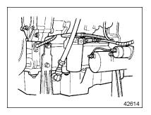
Figure 17 Spin-On Fuel Filter Location
