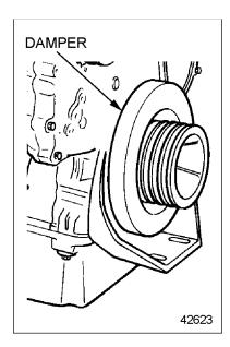
Figure 21 Viscous Vibration Damper
