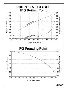
Figure 27 Coolant Temperatures vs. IPG Concentration (Sea Level)
