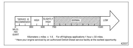
Figure 11 Engine Oil Consumption Guidelines
