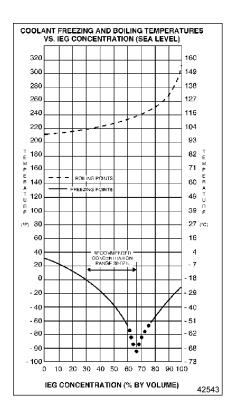
Figure 26 Coolant Temperatures vs. IEG Concentration (Sea Level)
