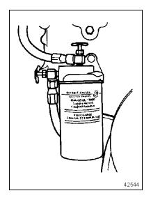
Figure 18 Coolant Inhibitor Element
