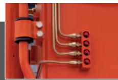
**Grouped greasing points** To simplify maintenance, the arm grease inlets have been grouped for easy access.
