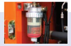
**Water separator** A highly efficient, high-capacity water separator protects the engine by removing most of the moisture from the fuel.
