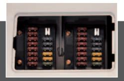
Convenient fuse box The fuse box is located in the storage compartment behind the seat, providing a clean environment and convenient access.
