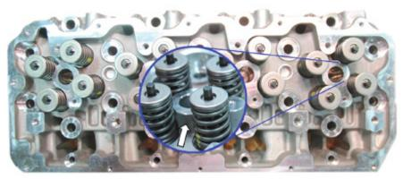
The third and final cylinder head (used from '06 MY-current) looks very similar to the second design cylinder head. The only distinct identifier is the glow plug hole, which uses a different thread so that it cannot be installed in the previous cylinder head.
