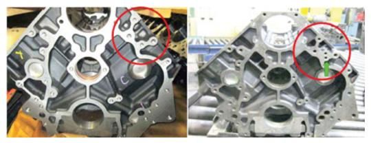
Figure 1. The block on left is 2001-'05 MY production and the block on the right is '06 MY and up production. Note the additional bolt holes for the later, higher-output water pump.
