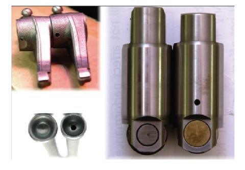
**Figure 5**. The upper left has the '05 MY on the left and '06 MY on right – note the difference in oil hole size. Pushrods on the lower left are '05 MY and earlier on the left and '06 MY and later on the right. Lastly, on the right side of the picture, the <u>cam follower</u> on the left is through '05 MY and '06 MY to current is on the right.
