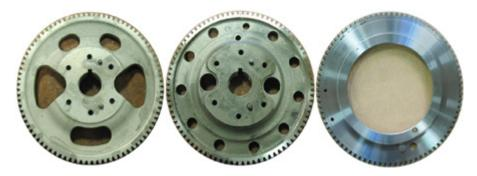
**Figure 4.** Camshaft timing gear on the left is early solid style thru '05 MY and on right the two pieces that are used as the spring loaded assembly to avoid and eliminate potential timing noise '06 MY to current.
