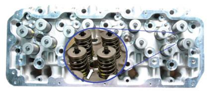
The second cylinder head, which came into being mid-'04 MY, had the revised valve cover and the new injector that was now outside of the lubricating oil (see **Figure 8**). This model head is easily recognized not only by the cover but the injector is longer and the mounting surface is a raised boss that you cannot mistake.
