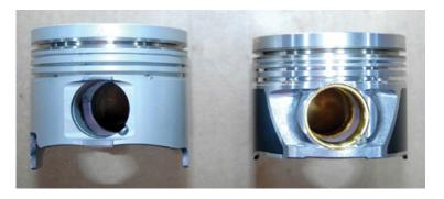
**Figure 6**. The piston on left was used up through the '05 MY and the piston on right is '06 MY and later with a longer wrist pin.
