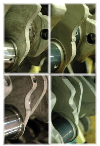
**Figure 3.** Upper and lower views on the left is the early crankshaft through '05 MY. The views on the right that have the small "bumps" in the forging are of the '06 MY to current production crankshaft. These crankshafts are balanced differently and are reported to be not interchangeable.
