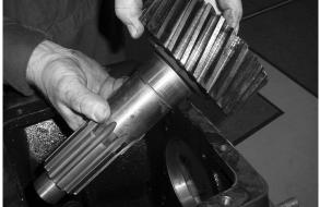
4. Move the drive gear forward to lightly tap the main bearing forward and out of the case bore.
