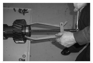
4. Remove the rear bearing from the countershaft.
