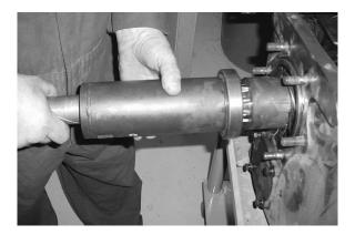
4. Install the outer bearing on the drive gear shaft, so it seats tightly against the spacer shield of the bearing to the front or facing away from the case.
