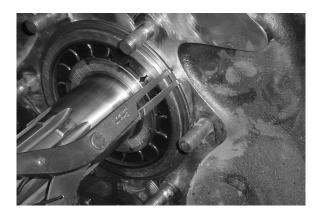
4. Install the snap ring into the groove in the bearing. Leave the drive gear in this position in order to provide space for installation of the mainshaft assembly.
