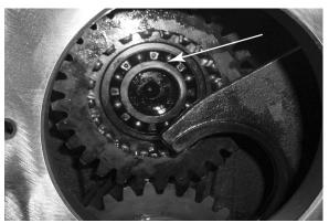
3. Install the mainshaft pilot bearing into the pocket of the drive gear.
