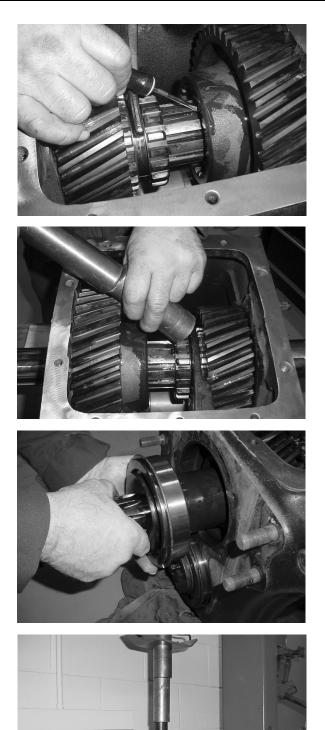
12. Inside the pocket of the low speed gear, turn the splined thrust washer in its groove until the lugs on its inside diameter line up with the grooves in the mainshaft.
