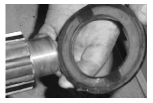
10. Continue to move the mainshaft forward in order to completely seat the pilot bearing on the front of the mainshaft, and at the same time move the sliding clutch gear back on the mainshaft.
