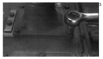
Install the retaining capscrews in the shift bar housing flange. Tighten to hold the assembly to the shift bar housing.
