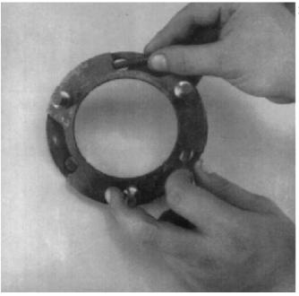
2. Install the 3 springs in the HI Range synchronizer ring bore.
