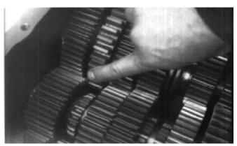
19. Mesh the upper countershaft marked timing tooth with the main drive gear two marked timing teeth, make sure the lower countershaft remains in time.
