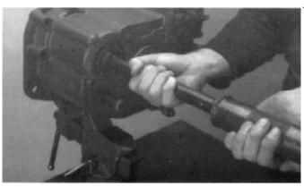
2. Remove the countershaft bearings from the auxiliary case bearing bores.
