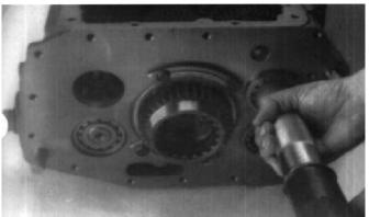
20. Hold the countershaft in position and partially install the rear countershaft bearing.
