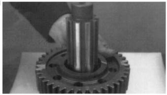
4. Install the LO Range gear rear washer on the output shaft and against gear, with the chamfer side facing up.
