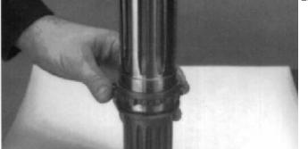
2. Place splined washer on the output shaft shoulder facing up as shown.
