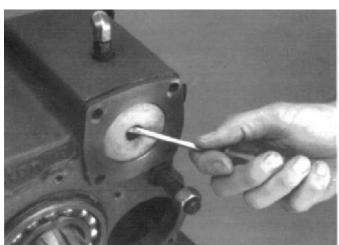
5. Remove the copper gasket from the yoke bar.
