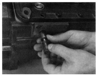
4. If necessary, remove the air line fittings from the slave valve.
