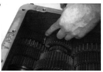
4. Install input shaft through case bore and into the drive gear splines. Installation of the input shaft prevents the mainshaft from dropping to the case bottom.
