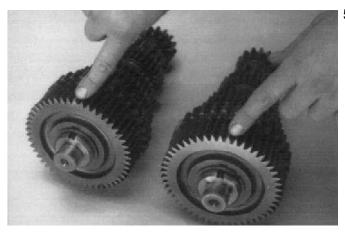
5. Install the snap ring in each countershaft front groove.
