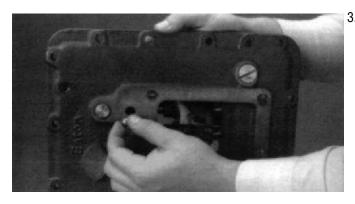
Tilt the assembly and remove the 3 detent balls from the housing bores.
