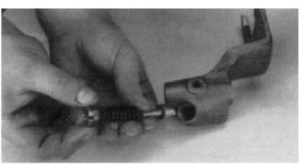
If previously removed, place plunger stop in 1st-reverse shift yoke block, install spring in bore of yoke and onto shank of plunger. Install the plug an tighten to compress the spring.
