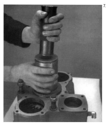
7. Install the bearing in the housing bore.
