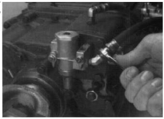
5. Install the Roadranger valve cover over the 2 air lines and gear shift lever. Install the jam nut on the shift lever. Thread the Roadranger valve on the shift lever and secure by tightening the jam nut against the Roadranger valve.
