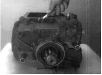
2. Install the 15 capscrews in the auxiliary housing flange and tighten to the recommended torque.
