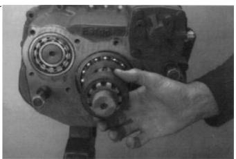
4. Remove the washer from the output shaft.
