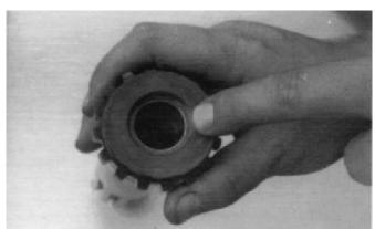
3. Mesh the lower countershaft marked tooth with either of the two marked teeth on the main drive gear.
