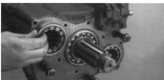
3. If necessary, secure assembly in a vice and remove the auxiliary countershaft front bearing race from the countershaft with a puller and bearing separator.
