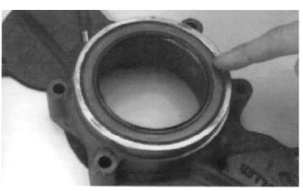
2. If necessary, remove the oil seal from the rear bearing cover.
