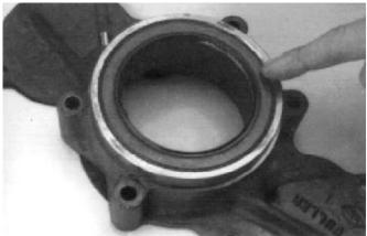
6. If previously removed, install the oil seal in the rear bearing cover, seal lip to the rear.
