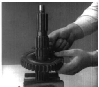
11. Remove the reverse gear and tolerance washer.
