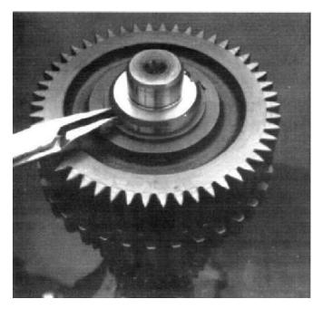
3. Remove countershaft drive gear, countershaft PTO gear, and countershaft 3rd speed gear together by pressing on the countershaft 3rd speed pear bottom face.
