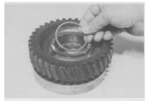
Figure 47 - Position roller spacer on first row of rollers.
