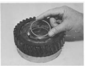
**Figure 49** - Position outer roller spacer on second row of rollers. Grease rollers to hold in place.
