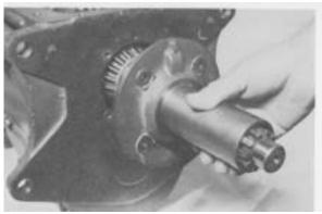
**Figure 159** - Position main drive gear bearing cap on main drive gear. Lube oil groove in cap at the top.
