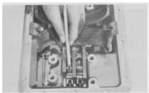
**Figure 131** - Note position of tapered interlock pins and shift rails.
