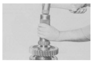
**Figure 66** - Using a suitable bearing driver and soft hammer install mainshaft rear taper bearing. Be certain bearing race is tight against split washer.
