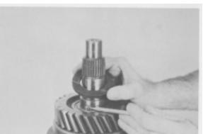
**Figure 44** - Install 3rd speed thrust washer lock ball, washer and washer retainer ring.
