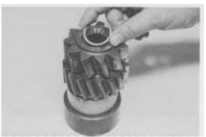
**Figure 148** - Position roller spacer on second row of rollers. Grease rollers to hold in place.
