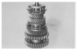
**Figure18** - Position mainshaft in a suitable stand. A vise may be used if soft jaw are utilized.
