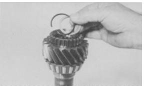
Figure 79 - Install roller bearing washer and retainer ring.
