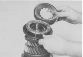
**Figure 73** - Install 4th & 5th synchronizer assembly and 5th speed synchronizer cup on shaft.
