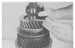
Figure 24 - Remove 3rd gear thrust washer. Use caution as NOT to lose lock ball.
