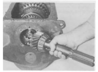
**Figure 157**- Remove transmission clutch housing. With main drive gear needle rollers in place and greased, position main drive gear in housing bore. Alogn clutching teeth on main drive gear with teeth in 5th speed synchronizer cup.
