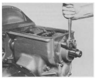
Figure 3 - Remove rear mainshaft bearing cap bolts.
