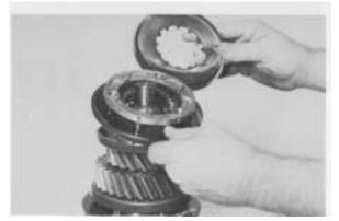
**Figure 19** - Remove 5th speed synchronizer cup and 4th & 5th speed synchronizer assembly.
