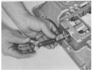
**Figure 118** - Remove reverse latch plunger spring and plunger.
