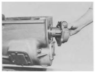
**Figure 4** - Remove rear mainshaft bearing cap and speedometer drive gear.
