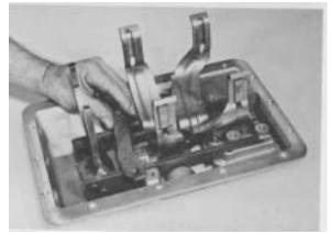
Figure 133 - Position rear rail support
