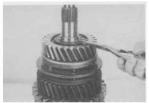
Figure 23 - Remove 3rd gear retaining ring.
