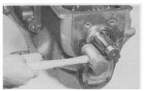
**Figure 154** - Using a soft hammer, tap rear bearing cup until cup locating ring is against housing.
