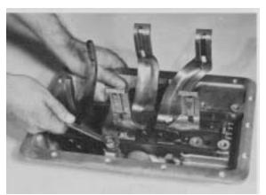
Figure 108 - Remove rear rail support capscrews.
