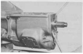
**Figure 5** - Tap on main drive gear to move mainshaft to the rear about 1/4" [6,35 mm]. Use pry bars as shown to remove rear bearing cup and locating ring.
