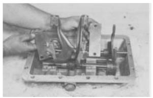
Figure 83 - Remove front and rear rail supports.
