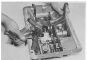
**Figure 111** - Remove 4th, 5th, 2nd & 3rd shift fork and rail assembly (See caution in Figure 112).
