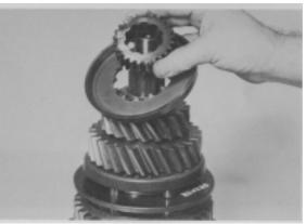
**Figure 21** - Remove 4th & 5th shift hub sleeve and 4th speed synchronizer cup.
