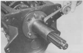
**Figure 162** - Recheck bearing capscrews and tighten to 30 inch lbs. torgue [3,4 N.m.].
