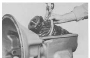
Figure 152 - Install mainshaft assembly into transmission case as shown.
