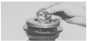
**Figure 74** - Grease thrust bearing and install bearing and bearing race on mainshaft.
