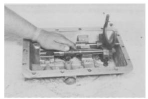
**Figure 98** - Install 1st & Reverse shift lug, rocker lug, shift rail and spacers in rail groove over mesh lock ball and spring. NOTE: Position widest spacer between shift lug and front support. (2) narrower spacers between the shift lug and center support.
