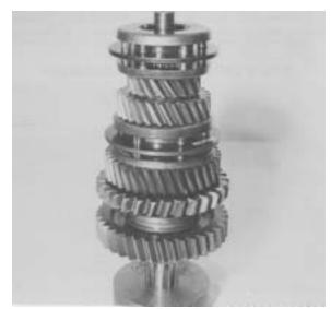
Figure 75 - Mainshaft assembly complete.
