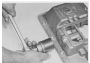
Figure 117 - Remove reverse latch plunger spring retaining plug.
