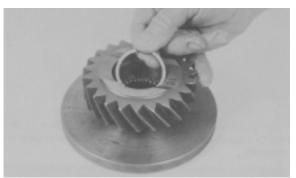
Figure 68 - Position roller spacer on first row of rollers.
