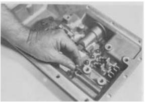
Figure 114 - Remove mesh lock poppet balls, quantity 4.
