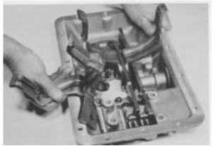
Figure 129 - Position 4th & 5th shift fork and rail on poppet ball in neutral.
