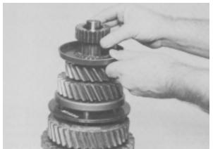
**Figure 72** - Position 4th gear synchronizer cup on clutching teeth of 4th gear. NOTE: Chamfer on I.D. of 4th & 5th shift hub sleeve must go down. Install shift hub sleeve on shaft.
