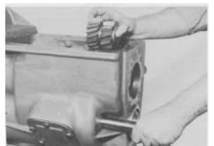
Figure 13 -Remove reverse idler gear and thrust washers.
