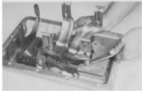
Figure 104 - Remove front rail support capscrews.
