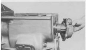
**Figure 155** - Coat O.D. of oil seal with Loctite 510 and press seal in mainshaft rear bearing cap with lip of seal down. Coat a new gasket on both sides with Loctite 510. Position gasket on mainshaft rear bearing cap. Use caution as not to cover oil return grooves in bearing cap. Install bearing cap with oil grooves lined up with oil holes in case.
