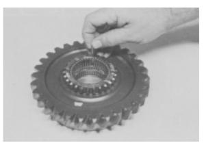
**Figure 57** - Lay up second row of needle rollers. Grease rollers to hold in place.
