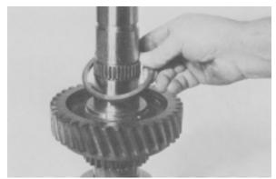
Figure 53 - Install split washer retainer ring over split washer.
