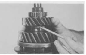
Figure 22 - Remove 4th speed gear. Use caution as NOT to lose needle rollers under gear. NOTE: Units built before serial number 045451YJ will not have needle rollers under 3rd & 4th speed main-shaft gears.
