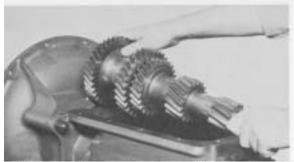
**Figure 139** - Tip rear of countershaft down and into transmission case. Feed rear of countershaft through rear countershaft bearing bore. Move countershaft forward and into pilot bearing. **CAUTION:** Do NOT disrupt countershaft needle bearing.
