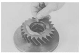
Figure 69 - Lay up second row of needle rollers.
