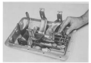
**Figure 135** - Install interlock tapered pin supports. Tap 4th & 5th shift fork to the rear. (4th speed position).
