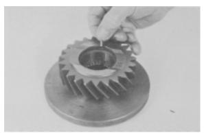
**Figure 67** - With clutching teeth of 4th gear down, coat inside diameter of gear with a high quality heavy grease. This will hold need rollers in position while assembling. Lay up first row of needle rollers.
