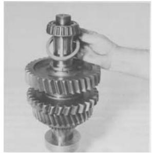
**Figure 29** - Remove rear bearing and split washer retainer ring.
