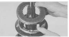
**Figure 26** - Remove 3rd gear synchronizer cup and synchronizer assembly. NOTE: There is a variation in the mainshaft 1st gear retention. One version has a split washer and a split washer retainer ring. Using a three-legged puller (as shown in Figure 27), pull against split washer retainer ring to remove rear bearing
