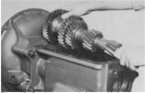
Figure 17 - Remove countershaft assembly from transmission case. Countershaft front pilot bearing has lose needle rollers. Use caution as NOT to lose these rollers.
