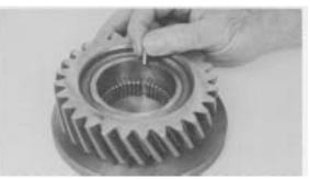
**Figure 38** - With clutching teeth of 3rd gear down, coat inside diameter of gear with a high quality heavy grease. This will hold needle rollers in position while assembling. Lay up first row of needle rollers.
