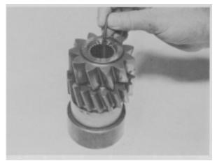
Figure 147 - Lay up second row of needle rollers.
