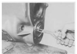
Figure 142 - Install countershaft rear bearing retainer ring.
