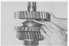
**Figure 31** - Remove 1st gear. Use caution as NOT to lose needle rollers under 1st gear. Ist gear was removed in Figure 28 for thrust washer retention. Further disassembly of the mainshaft will be identical in both versions.
