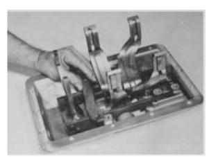
Figure 109 - Remove rear rail support.
