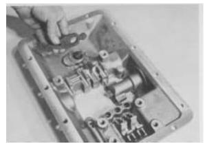
Figure 116 - Remove 1st & Reverse rocker arm.
