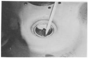
**Figure 138** - Coat countershaft pilot bearing needle rollers with heavy grease to hold in place until countershaft is installed.
