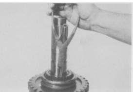
**Figure 32** - Remove 1st & Reverse shift hub sleeve retainer ring.
