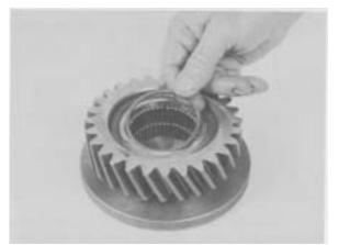
Figure 41 - Position outer roller spacer on second row of rollers. Grease rollers to hold in place.
