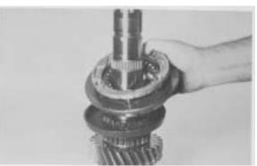
**Figure 45** -Turn mainshaft over. Install 3rd gear synchronizer cup and 2nd & 3rd synchronizer assembly.
