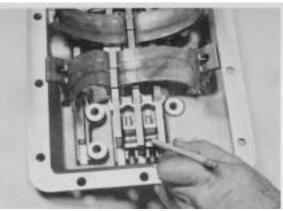
**Figure 107** - Note position of interlock tapered pins for reassembly.
