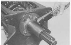
**Figure 160** - Install two capscrews 180 Degrees apart and torgue screws to 15 inch lbs. [1.7 N.M.].
