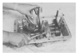
Figure 82 - Remove front and rear rail support capscrews.
