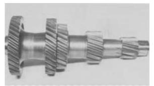
**Figure 80** - If the countershaft, drive gear or 4th gear is to be replaced (Figure 80 shows direction of drive gear and 4th gear hubs).
