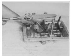
**Figure 102** - Tighten support capscrews 20 - 25 ft.lbs. torque [27,2 - 33,8 N.m].
