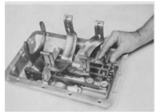
Figure 106 - Remove interlock tapered pin supports.
