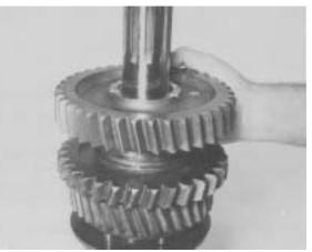
**Figure 62** - With clutching teeth of 1st gear down, follow same procedure used in Figures 54 thru Figure 57 to install needle rollers and spacers. Install 1st gear on mainshaft.
