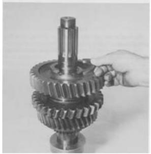
Figure 30 - Remove 1st gear split washer
