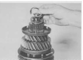
**Figure 20** - Remove shift hub thrust bearing and bearing race.
