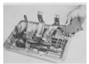
Figure 105 - Remove front rail support.
