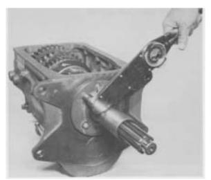
**Figure 166** - Install capscrews and tighten 15 - 20 ft.lbs. torque [20,4 - 27,1 N.m.].
