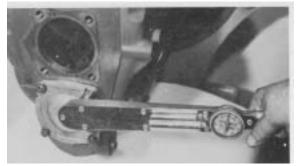
**Figure 151**- Coat a new gasket on both sides with Loctite 510. Position gasket on countershaft bearing cap. Install bearing cap and bolts. Tighten bolts 20 - 25 ft.lbs. torque [27,2 - 33,8 N.m.]
