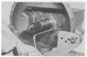
Figure 6 - Remove main drive gear cap bolts.
