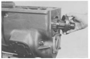
**Figure 153** - Position mainshaft rear bearing cup in housing bore.
