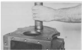
**Figure 81** - If countershaft front bearing is to be replaced, remove clutch housing and drive front bearing from transmission case. Apply a light coat of Loctite 510 on the outer diameter of the new bearing. Install in transmission case as shown with end of bearing .001-.007 below the face of case. Clutch housing is reassembled temporarily on transmission case to facilitate reassembly of transmission, but will be removed again later on to set mainshaft taper bearing end play.
