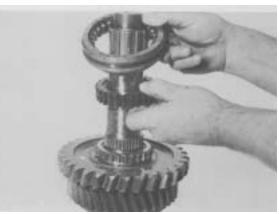
Figure 33 - Remove shift hub and sleeve.
