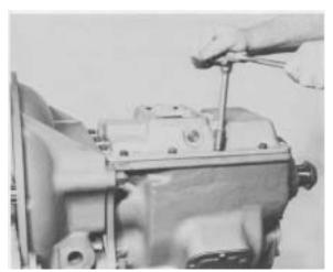
Figure 2-Remove control cover capscrews and control cover.
