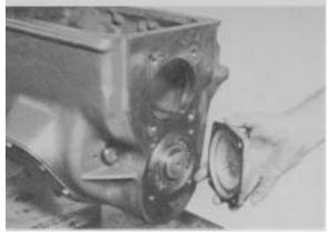
Figure 11 - Remove countershaft rear bearing cap.
