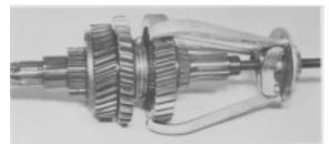
**Figure 28** - Remove rear mainshaft bearing and 1st gear, as shown. Use caution as NOT to lose needle rollers under 1st gear. (See Note after Figure 26).
