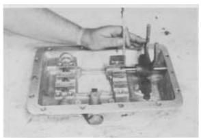
**Figure 87** - Using a small magnet, remove the 1st & Reverse shift fork rod lock pin.
