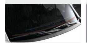
Wiper de-icer A heating element embedded in the lower windscreen melts away ice and frees up frozen wipers.
