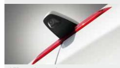
LED stop lamp and rear camera Roof mount gives maximum camera scope and stop visibility. Boosting safety.
