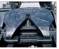
High-Height Coupler Featuring pitch and roll movement, the dual-axle coupler is available on HD700 and HD1000. Robust designs of coupler offer outstanding shock-absorbing characteristics
