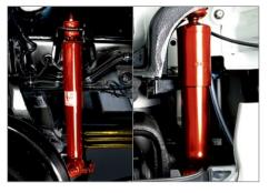
Shock Absorber New hydraulic dampers improve steering and handling qualities for a more precise and comfortable driving.
