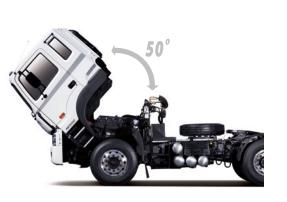
▲ 50-Degree Tilting Cab Service personnel will appreciate the extra-wide cab tilting angle which makes it easy to access the engine to perform maintenance and repair work.
