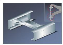
**Crossmember Reinforcement** To achieve the highest possible rigidity and strength of frame for distributing payload, heavy duty crossmembers are added using all bolted construction technique.
