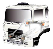
Coil Type Full Floating Cab Suspension ► The cab rides on four coil spring mounts to free the driver from fatigue road shocks and vibration. An air suspension provides an option.
