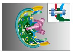
**Wheel Hub Pilot** The hub pilot on wheel is designed to optimize torque of the lock nuts and eliminate vibration for safer driving.
