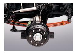
**Tapered Leaf Spring** The spring mass of the front axle is reduced by the application of long tapered parabolic springs which improve load distribution and maximize load carrying performance. Hydraulic dampers fine-tune performance.
