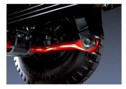
Front Stabilizer Bar Front stabilizer bar increases structural rigidity to more effectively absorb vibration and road shocks.
