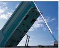
Telescopic-type (HD370) dump mechanism
