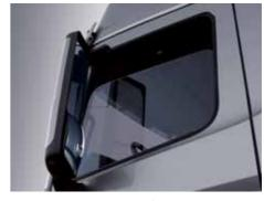
Pull-down door glass (Application of water-repellent door glass)
