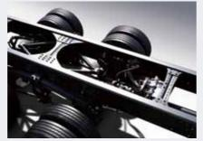
Front frame & High-tensile chassis
