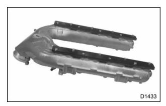
Figure 104 Test plates installed on intake manifold
