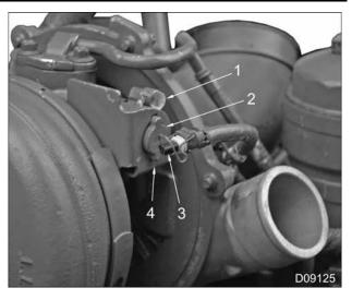
Figure 46 Disconnection of VGT control valve
