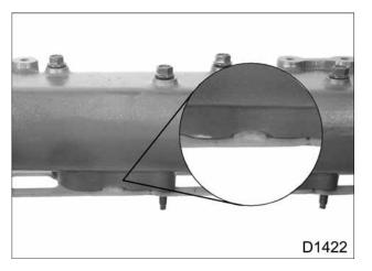
Figure 113 Intake manifold gasket with centering tab
