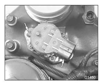
Figure 90 EGR valve retaining bolts
