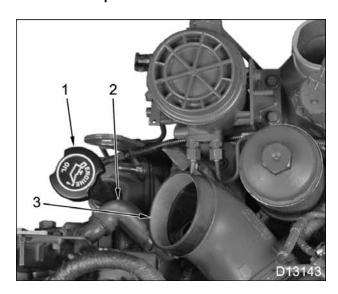
Figure 49 Air inlet duct
