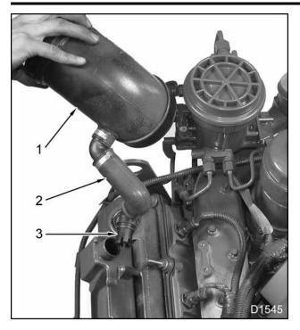
Figure 51 Breather tube and pitot tube
