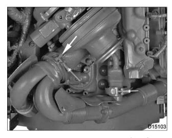
Figure 69 Exhaust adapter V-clamp for VGT
