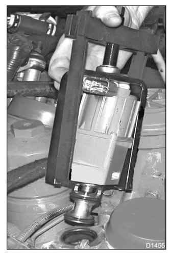
Figure 94 EGR valve removed
