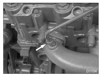
Figure 85 Tube fitting for EBP sensor
