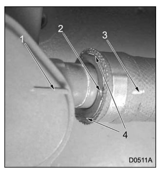
Figure 118 EGR coolant inlet coupling alignment (unlocked position)
