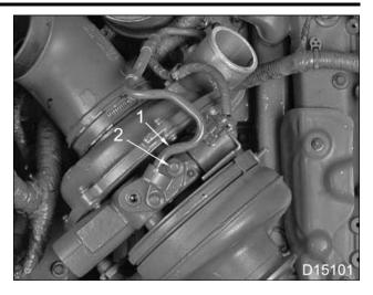
Figure 52 Oil supply tube to VGT
