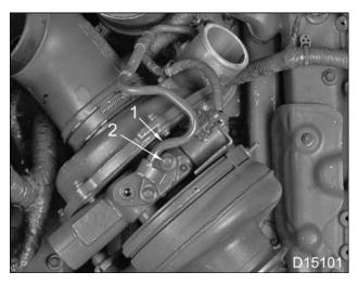
Figure 72 Oil supply tube for VGT
