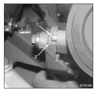
Figure 68 VGT alignment dowels and bosses
