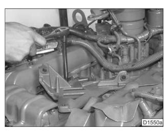
Figure 61 Removal of VGT bracket bolts
