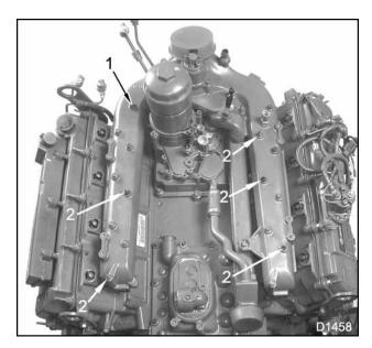
Figure 96 Dog point bolts stud bolts
