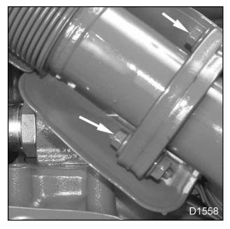
Figure 126 Exhaust tube bolts (upper right)
