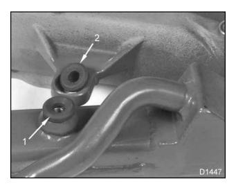
Figure 109 Bosses between EGR cooler and intake manifold
