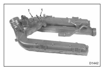
Figure 108 EGR cooler retaining bolts
