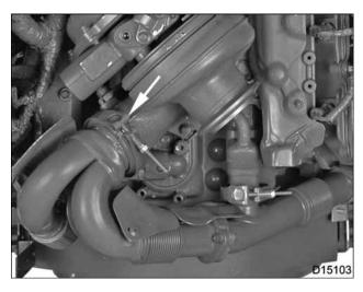
Figure 54 Exhaust adapter V-clamp for VGT
