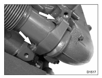
Figure 122 Mounting bolts for right exhaust tube
