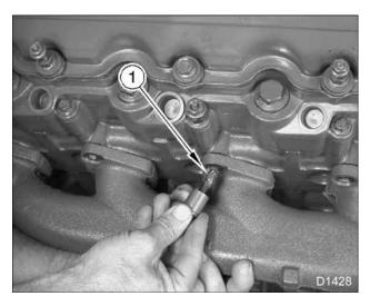
Figure 124 Bolt and spacer for left exhaust manifold
