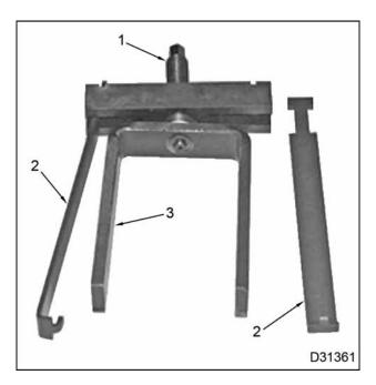
Figure 92 EGR Valve Puller
