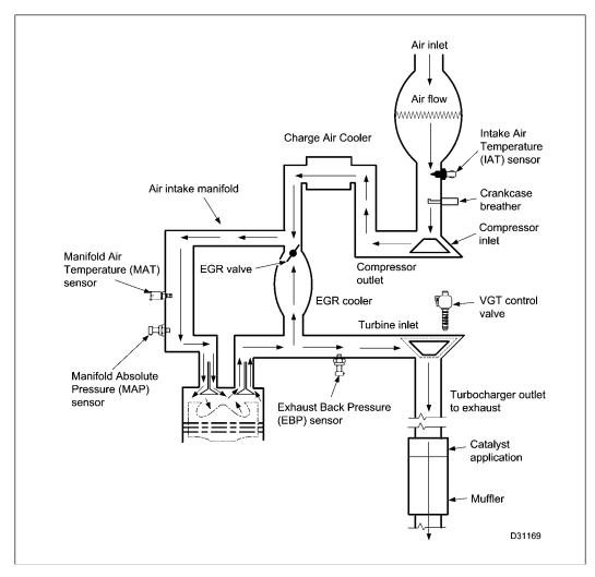
Figure 12 Air flow diagram
