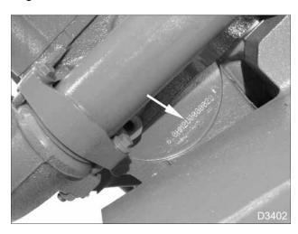
Figure 1 Engine serial number
