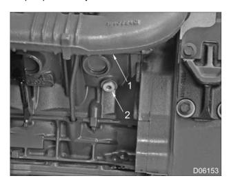
Figure 41 Left side coolant drain plug
