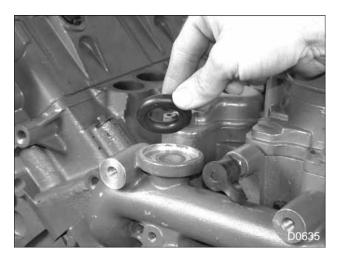
Figure 112 Front module seal
