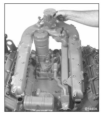
Figure 100 Intake manifold and EGR cooler
