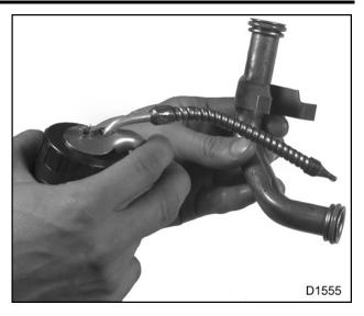
Figure 67 Lubrication for O-rings on oil drain tube for VGT
