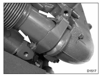
Figure 87 Right exhaust tube assembly
