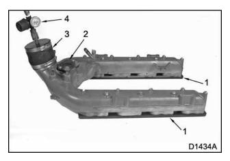
Figure 105 Set up for intake manifold pressure test
