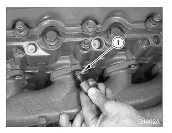
Figure 120 Right exhaust manifold bolt and spacer
