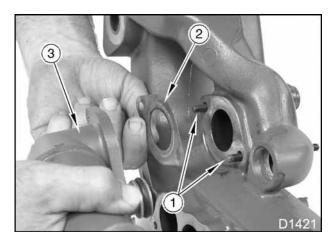
Figure 107 EGR cooler connection to intake manifold
