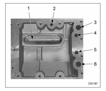
Figure 30 Oil reservoir in crankcase
