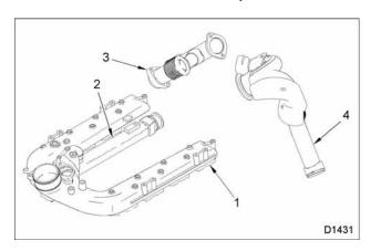
Figure 81 Exhaust Gas Recirculation Components (EGR)
