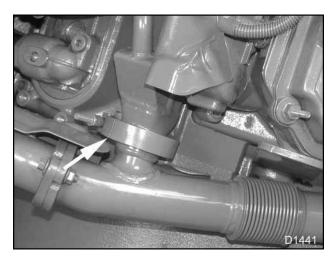
Figure 123 EGR cooler V-clamp
