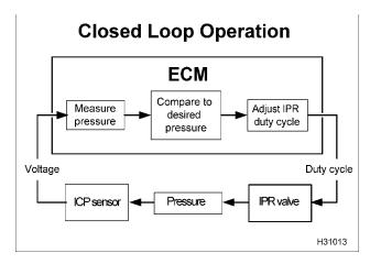
Figure 22 ICP closed loop system
