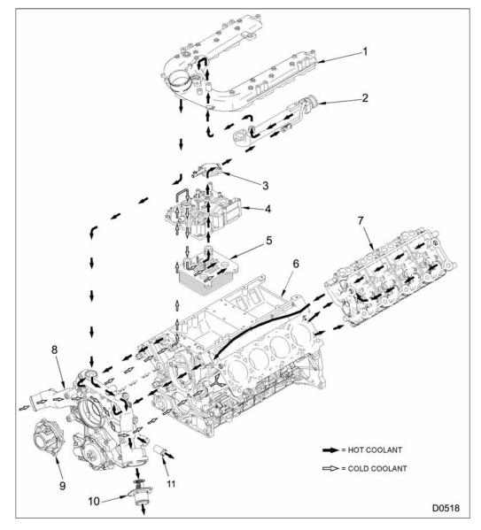
Figure 31 Engine cooling system components
