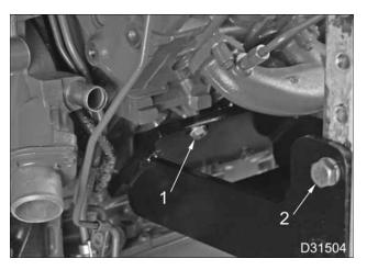
Figure 44 Mounting bolts for Engine Stand Mounting Bracket
