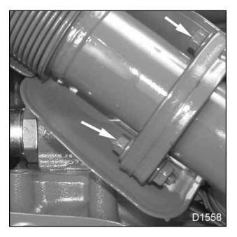
Figure 84 Exhaust tube bolts (upper right)
