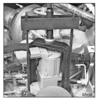
Figure 93 EGR valve puller installed
