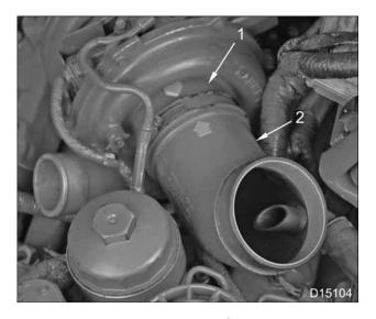
Figure 74 Air inlet duct to VGT
