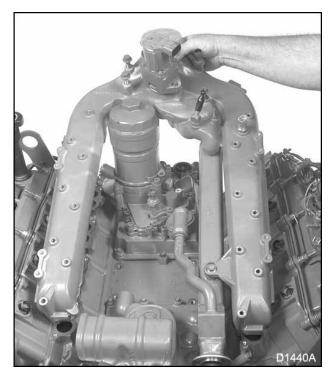
Figure 114 Intake manifold and EGR cooler assembly
