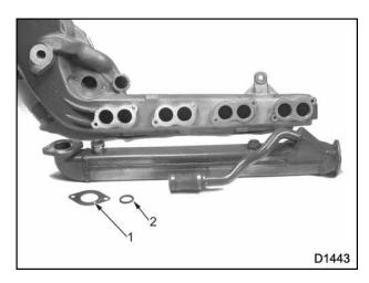
Figure 102 EGR cooler assembly
