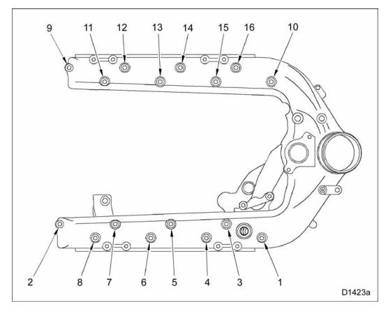
Figure 116 Torque sequence for intake manifold mounting bolts
