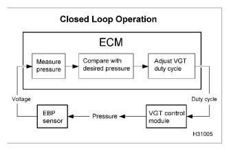
Figure 15 VGT closed loop system
