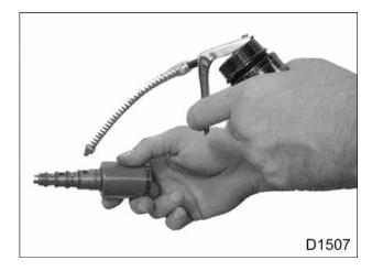
Figure 76 O-ring lubrication
