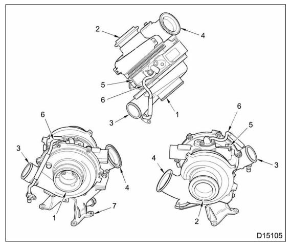
Figure 45 Turbocharger components
