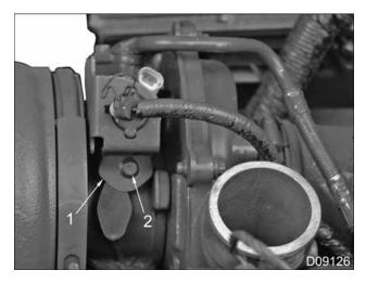
Figure 78 Retaining bolt for VGT Control valve
