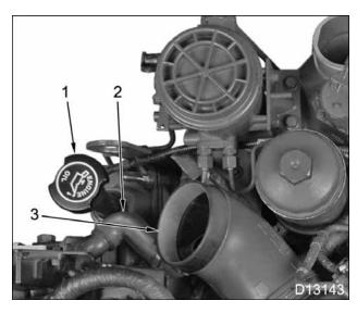
Figure 75 Air inlet duct
