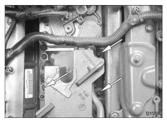
Figure 60 VGT bracket bolts
