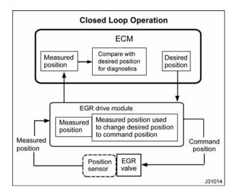
Figure 19 EGR closed loop operation
