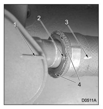
Figure 97 EGR coolant inlet coupling
