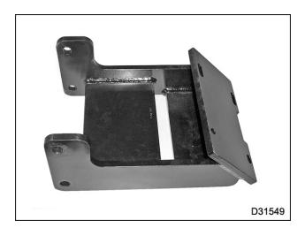
Figure 43 Engine Stand Mounting Bracket
