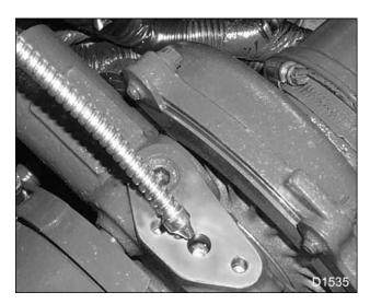
Figure 71 Prelubrication of VGT bearings
