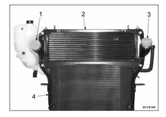
Figure 13 Charge Air Cooler
