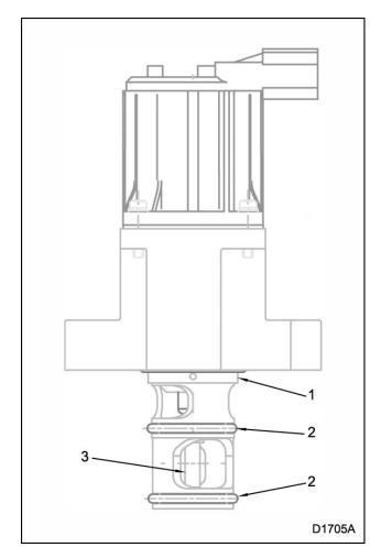
Figure 103 EGR valve assembly
