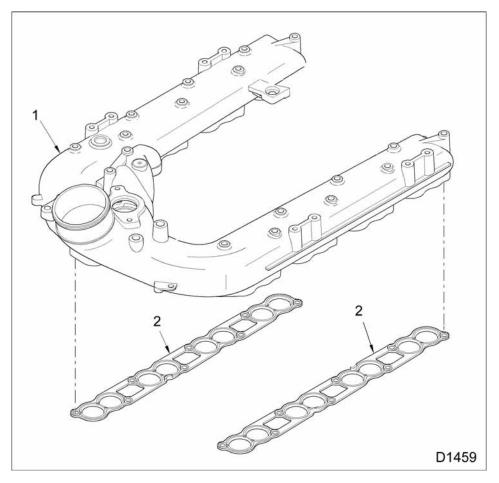
Figure 80 Intake manifold and gaskets
