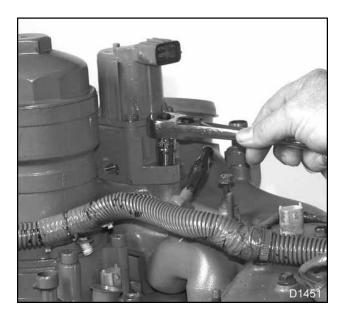
Figure 91 EGR valve retaining bolts
