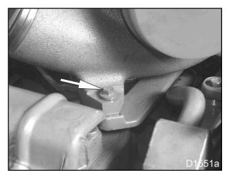
Figure 56 Rear mounting bolt for VGT
