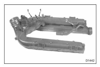
Figure 101 EGR cooler retaining bolts
