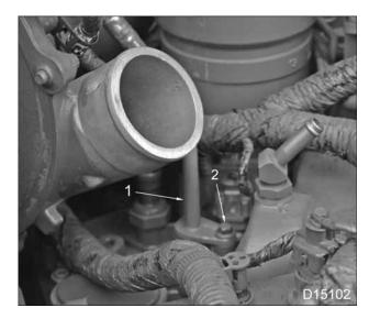
Figure 53 Oil supply tube for VGT to oil cooler cover assembly
