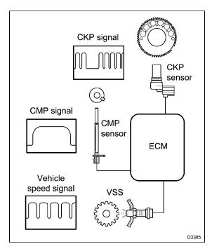
Figure 37 Magnetic pickups
