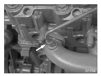
Figure 125 EBP sensor tube fitting
