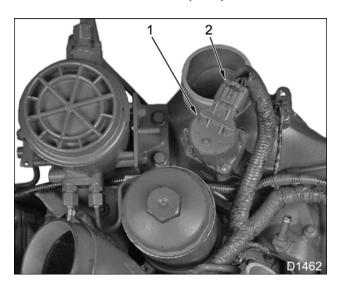
Figure 89 EGR valve and 8-pin electrical connector
