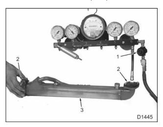
Figure 106 EGR cooler with pressure test plates installed
