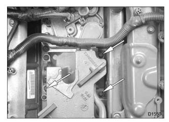
Figure 66 VGT bracket bolts
