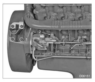
Figure 42 Right side coolant drain plug
