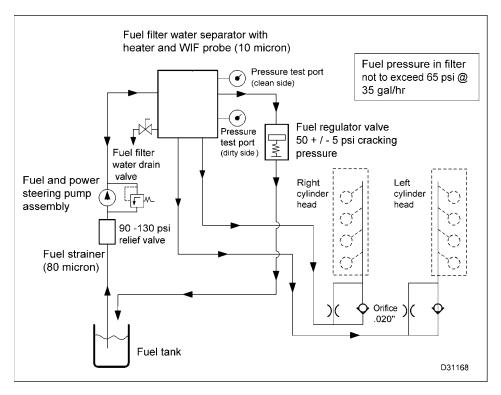
Figure 26 Fuel system schematic
