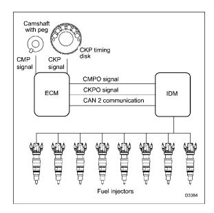
Figure 33 Injection Drive Module (IDM)
