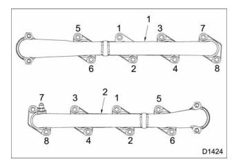
Figure 121 Torque sequence for exhaust manifold mounting bolts
