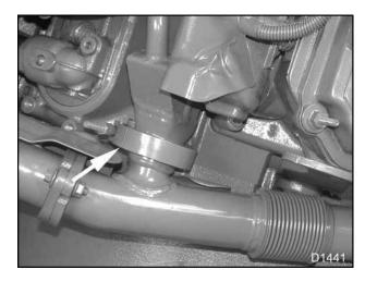
Figure 99 V-clamp on EGR Cooler
