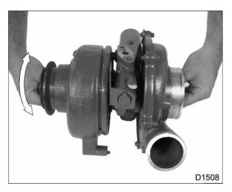
Figure 63 Free rotation of VGT shaft
