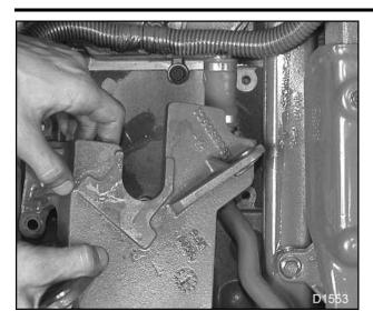
Figure 62 VGT mounting bracket
