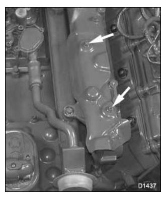
Figure 117 Heat shield mounting nuts (right side)
