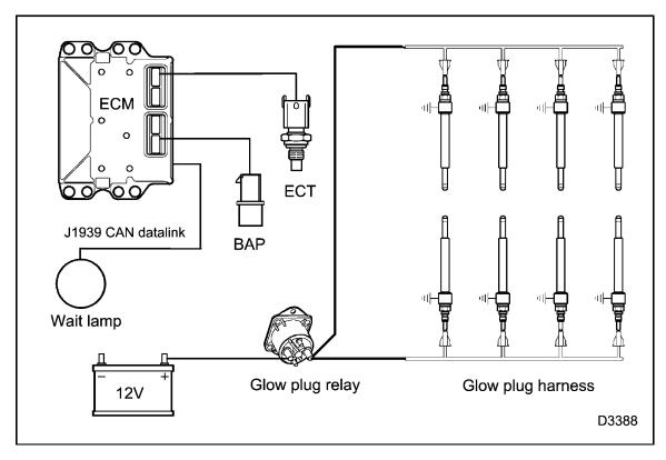
Figure 40 Glow plug control system
