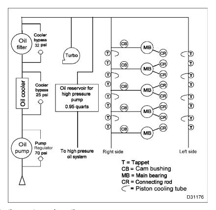
Figure 28 Lubrication system schematic
