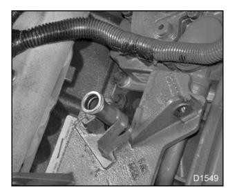
Figure 58 Oil drain tube for VGT
