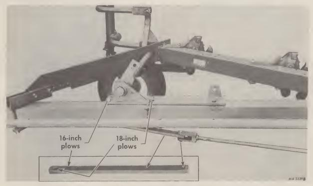
Illust. 28A - Locate and secure tie rod for 16-inch and 18-inch plows as shown.
