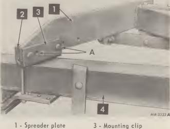
2 - Spacer 4 - Pull beam Illust. 14B - Six Furrow Plow.
