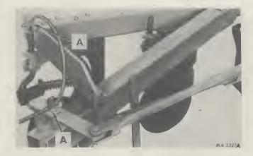
Illust. 25B Install front hose supports as shown at ''A''.
