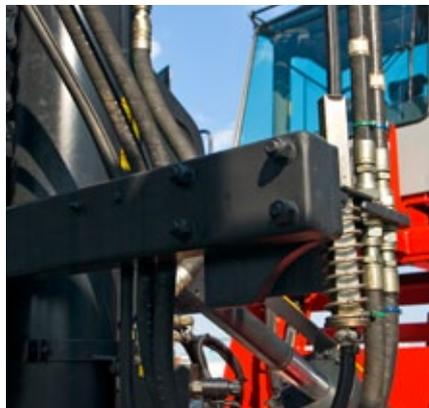
*Fewer components makes for increased reliability, only two hoses and one harness runs over the mast wheel.*
