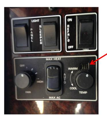
Have voltmeter in C77 SU wire and to ground, to check voltage change when blowing on Temp sensor
