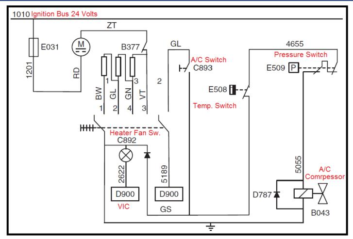
The Compressor is energized by VIC via Temperature Switch and Pressure Switch . The VIC communicates with the engine ECU via V-CAN, and will de-energize the A/C circuit (GRA5189-0) when coolant temp goes above 216°F (102°C) and reenergize it when coolant drops below 208°F (98°C).
