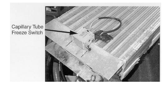
Both B-Cab and T2000 trucks use a freeze switch in the ground side of the HVAC relay control circuit
