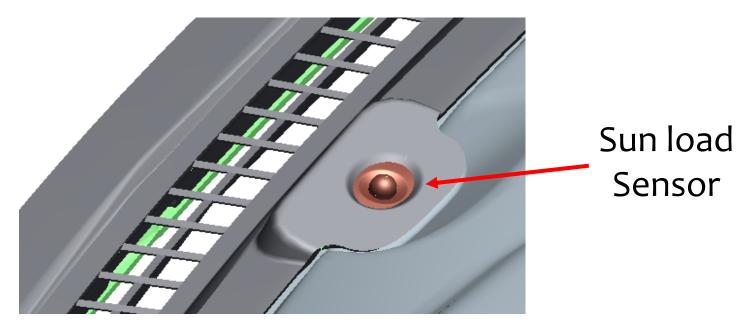
Sensor resistance across pins A and B is 150K to 190K with no direct sun light
