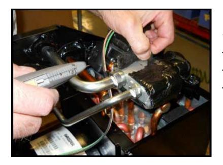
If there is a brass set plug with two drilled removal tool holes, **replace the expansion valve**.
