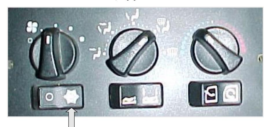
A/C switch on the left side of the control panel
