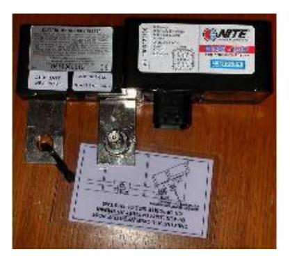
This device monitors the auxiliary batteries for state of charge, communicates with the KIM system and controls the battery separator solenoid.
