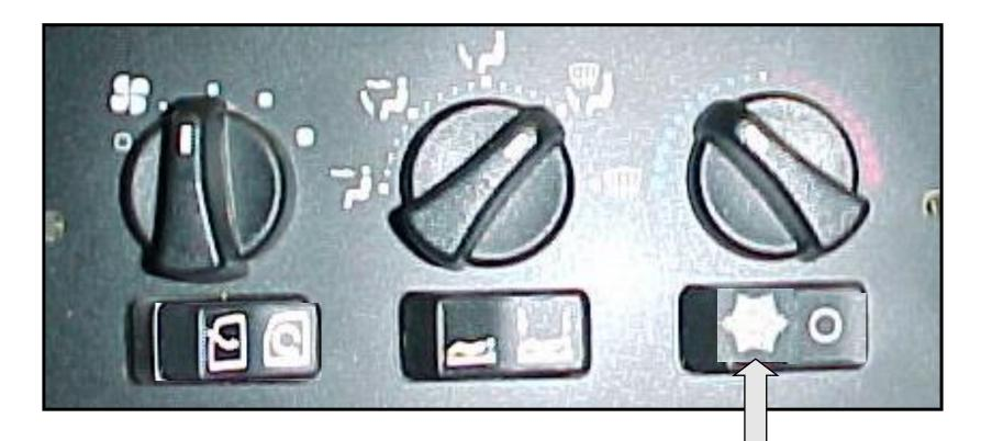
A/C switch on the right side of the control panel
