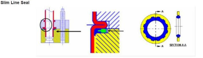
Per Parker Engineering (manufacturer of the seals), these are not to be lubricated during installation.
