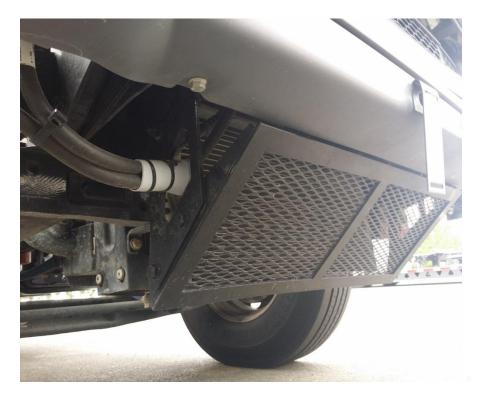
Note: Due to the low mount design of the condenser, road debris buildup inspection is an initial diagnostic step
