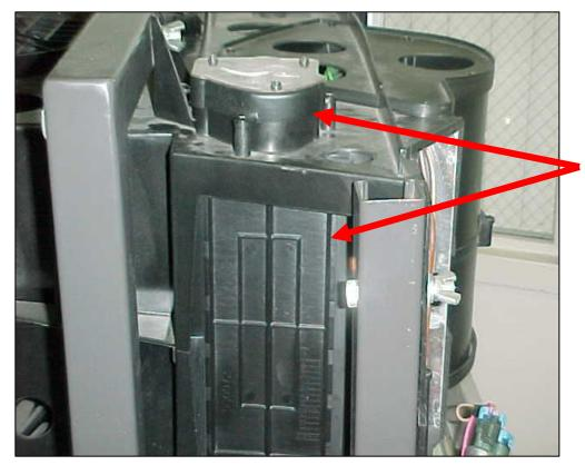
T2000 - uses an electric actuator to control fresh air door using voltages of 12V and <1V
