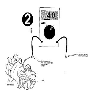
Measure available voltage at the clutch (SYSTEM VOLTAGE or above 11.5 volts)
