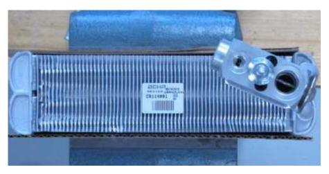
Finished Position of TXV Relative to Evaporator after Torque Applied
