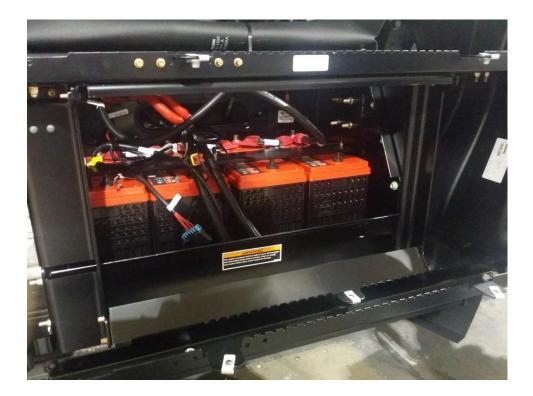
The four auxiliary batteries are installed in the passenger side step assembly. This may relocate the SCR & DPF assemblies to the area between the frame rails.
