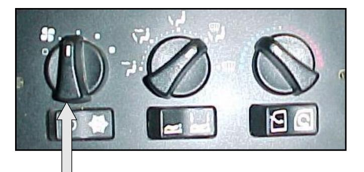
The T2000 has the cab blower circuit wired up as ground side switching and sleeper blower circuit is the opposite - power side switching.
