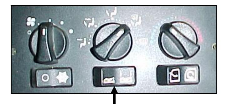
The Sleeper Rocker Switch controls power to the Sleeper Control Panel through circuit number P124SHA.
