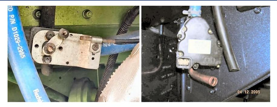
Kenworth utilizes hot water valves in many HVAC systems, with two basic types: Cable operated and Electronic
