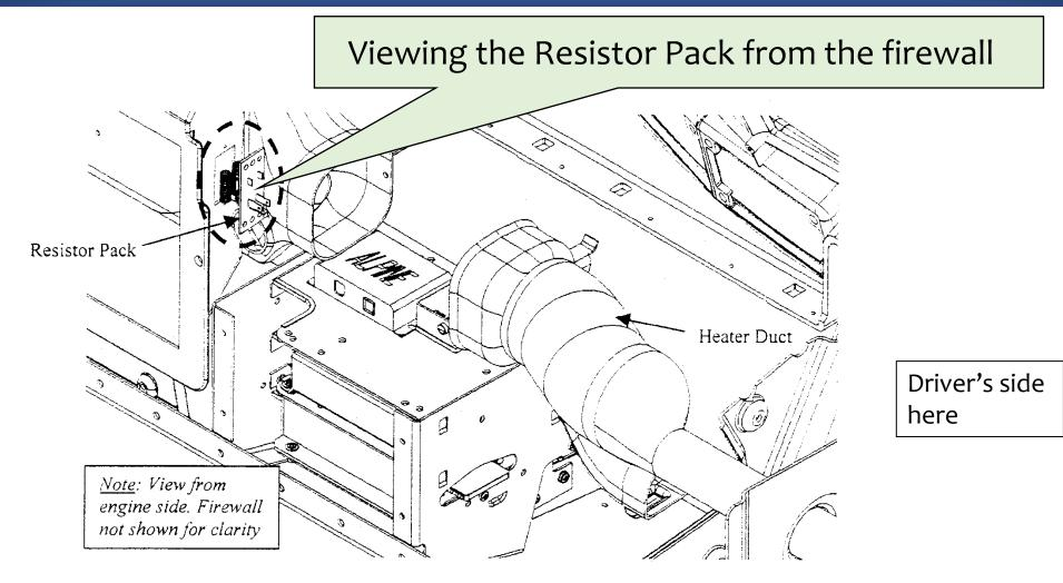
\* Must remove cup holder to get at resistor pack. Slide heater duct towards Driver's Side
