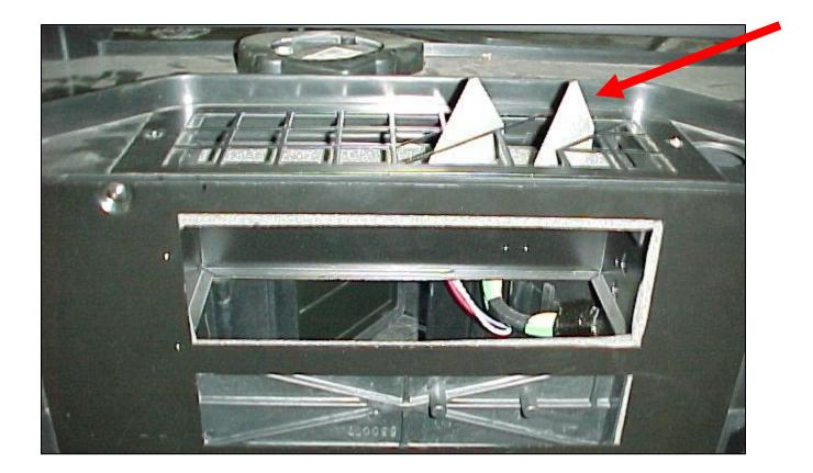
Put unit into defrost mode before removing unit from under dash, as the tabs will be damaged during removal otherwise.
