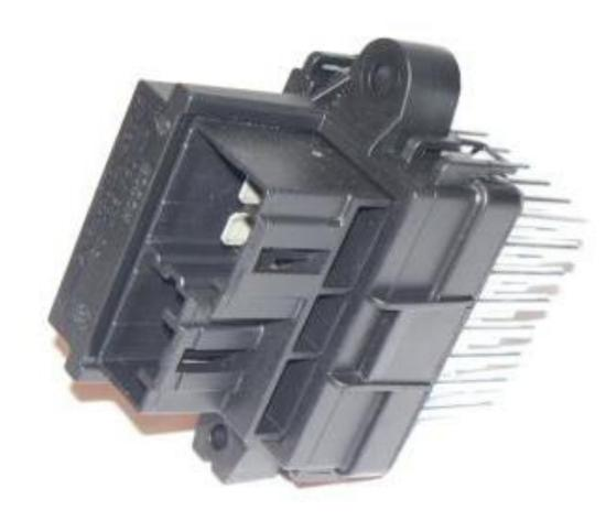
This module controls the amount of voltage delivered to the evaporator blower creating variable blower speeds. It is located in the return air in front of the evaporator coil.
