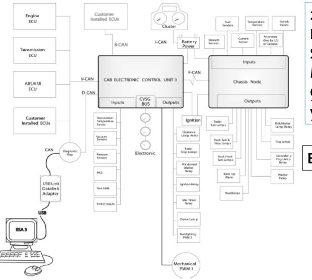
2010 Multiplexed Electrical System Service Manual — <u>CECU3</u> w/Chassis Node
