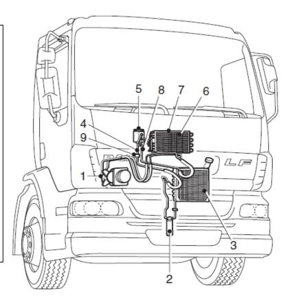
The air conditioning system is a closed system filled with R134a refrigerant. The A/C Includes a 24V Compressor.
