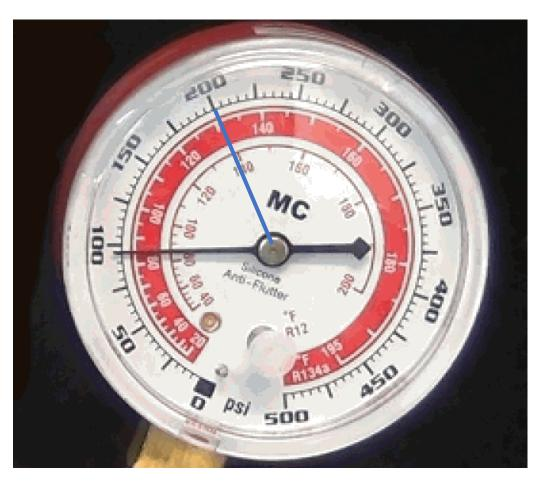
Many refrigerant gauge sets have an inner scale that reads the saturation (boiling) point of the refrigerant.
