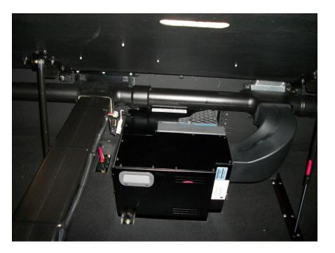
The main unit resides under the sleeper bunk and contains the system's evaporator, blower, compressor and the air filter.
