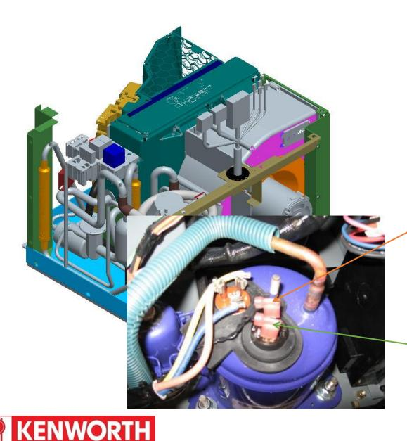
Compressor uses PVE oil only. Never contaminate with PAG oil
