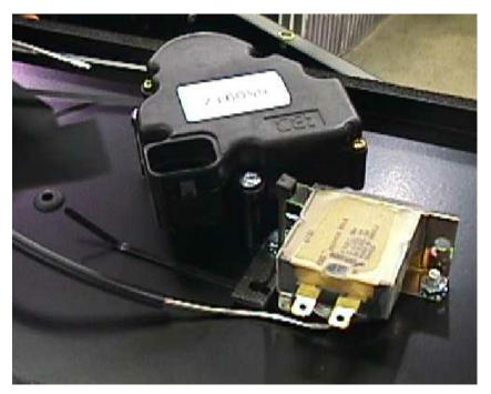
Both B-Cab and T2000 use the freeze switch in the ground side of the HVAC relay control circuit. The freeze switch opens at **31.5° F** and closes at **40°F**.
