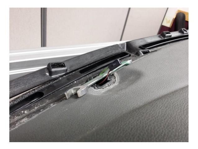
Secure sensor wiring harness connector to prevent it from falling down into the dash!
