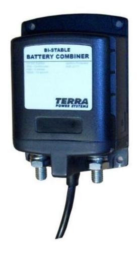
This device connects the truck batteries to the Aux batteries. When the starting batteries are at or above 13.2 volts, the battery management device will engage the solenoid to allow the alternator to charge the auxiliary batteries.
