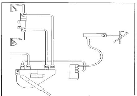
Early B-CAB uses a pneumatic pressure system for door and vent controls
