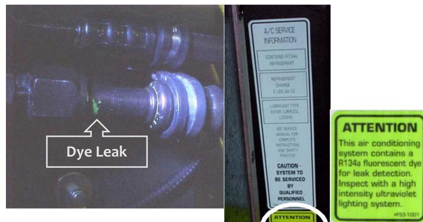
Dye wafer - Factory Installed since 10/29/01
