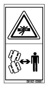
Sign indicates a crush hazard between the articulating parts of vehicle.
