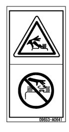
Sign indicates a burn hazard from spurting hot water or oil if radiator or hydraulic tank is uncapped while hot.
