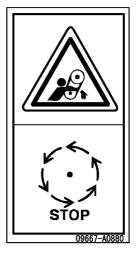
Sign indicates a hazard of rotating parts, such as belt.
