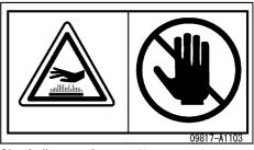
Sign indicates a burn hazard from touching heated parts, such as engine, motor, or muffler during or right after operation.
