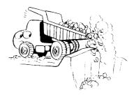
Never drive with the dump body raised. Always lower the body before moving.
