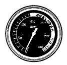
The tachometer indicates the engine speed in revolutions per minute. When the pointer enters the red range, it indicates that the engine is over running. The tachometer should not be allowed to enter the red range by braking the running speed.
