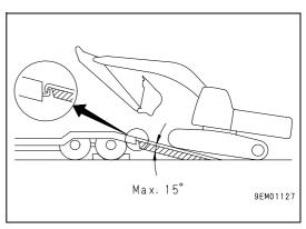
During the loading and unloading operations, always use ramps or a platform and proceed as indicated below.
