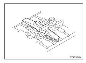
If the rubber track cannot be tensioned correctly through the injection of grease, check the track tensioner gaskets and if necessary change them or even the track. (See "4.9.1.g CHECKING AND ADJUSTING THE RUBBER TRACK TENSION").
