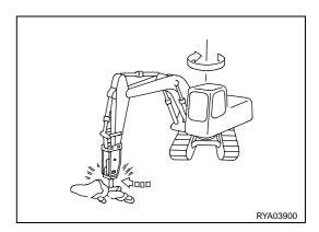
3. Moving the tool while it is hitting the material to be broken.
