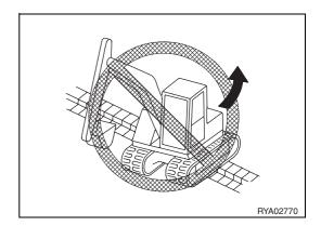
2. When travelling up slopes in reverse, avoid steering at the beginning of the slope. If it is necessary to steer on a slope, carry out this manoeuvre gradually.
