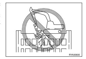
When carrying out demolition work, do not position the machine under the structure being demolished, since broken parts may fall down or the building may collapse causing serious injury or property damage.
