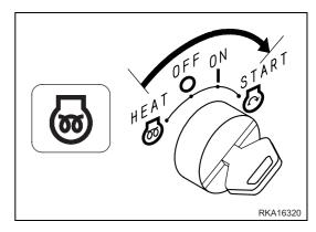
5. As soon as the engine starts, release the key (3), which will automatically return to position ON.
