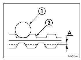
When the steel core is visible in two or more points of the track.
