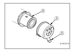
5. Slightly strike the filtering element (4) on the palm of your hand, in such a way as to remove the dust, and blow compressed air on the inner surface, keeping the air jet at a distance of approximately 15 cm and the pressure below 4-5 bars.
