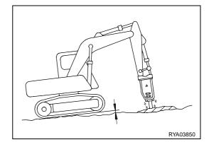
3. When working on very hard materials it is important to avoid hitting the same point for more than 30 seconds.
