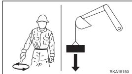
3 - MOVE THE LOAD AWAY IN HORIZONTAL DIRECTION With an arm extended forwards and the hand in vertical position directed towards the load to be moved away, move the hand in the direction of the movement to be carried out.
