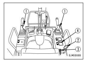
1. Make sure that the safety lever (1) is in the "locked" position (L). If the safety lever is in the "free" position (F), the engine cannot be started.
