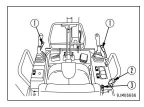
Make sure that the safety lever (1) is in the "locked" position (L). If the safety lever is in the "free" position (F), the engine cannot be started.
