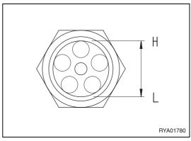
4. Extend the boom, arm and bucket cylinders completely, as shown in the diagram on the right, and remove the filler cap. Put back the cap and pressurize the tank, lowering the equipment to the ground.
