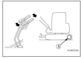
• When the sprocket (A) is at the front of the machine, push the levers (3) slowly forward to start moving in reverse.
