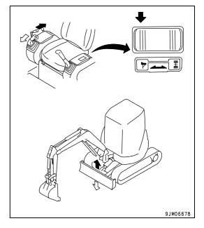
• Track gauge adjustment control (version with adjustable track gauge)
