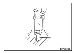
6. Hitting the ground with the breaker bit.
