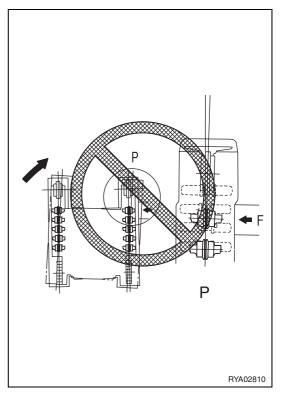
• If the machine travels in reverse in these conditions, the rubber track will come off.
