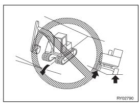
4. If the machine is operated in the conditions described in points from 1 to 3 above, do not change direction if the tracks do not adhere perfectly to the ground, see figure.
