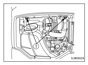
• Make sure that the cab floor is properly fastened with the screws (1). If it is not secured properly, it may cause serious injury.
