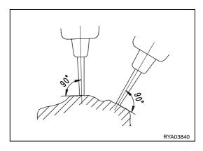
2. It is absolutely necessary to keep the pressure of the excavator on the breaker constant as the bit penetrates the ground.
