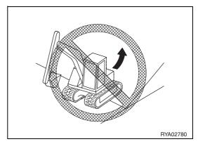
3. Do not proceed along the edges of a slope or on uneven ground keeping one track in horizontal position and the other inclined or partially raised (with machine inclination exceeding 10°C). To avoid damaging the rubber tracks, always proceed with both tracks resting on the same horizontal plane.
