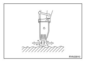
4. Working with the breaker in horizontal position or even more inclined.
