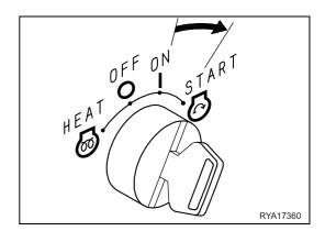
4. As soon as the engine starts, release the key (3), which will automatically return to position ON.
