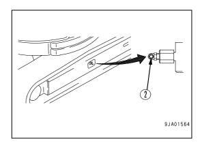
When after the injection of grease the idler roller sliding plate reaches the measure «S» of 0 mm and the track is not sufficiently stretched, this means that the pins and bushings are excessively worn. Therefore, it is necessary to exchange or replace the pins and bushings.
