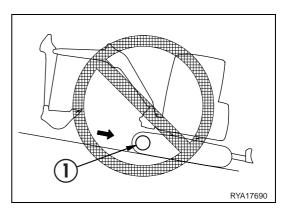
2. When travelling uphill on a slope whose inclination exceeds 15°, position the work equipment as shown in the diagram on the right.
