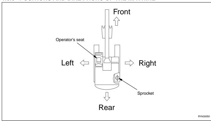
In this manual, the terms front/forward, rear/backward, left, and right refer to the travel direction as seen from the operator seat when it is facing the front and the sprocket is at the rear of the machine.
