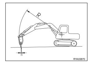
5. Always make sure that the thrust is optimal, in order to avoid dangerous and useless strokes.
