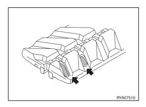
3. When more than half of the steel core cords at the centre of the track are cut.
