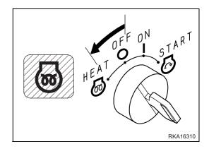
4. When the preheating warning light (4) goes out, turn the ignition key (3) directly to position START to start the engine.
