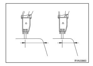
4. To facilitate the sliding of the tool on its seat, check the thrust direction and always correct the hitting position of the breaker using the bucket and arm control.
