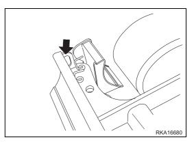
8. Install one shackle in the lifting hole provided in the boom, then pass the metal cable through it.
