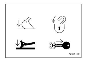
2 - Engage the safety locks of the boom swing, optional equipment and turret swing controls.
