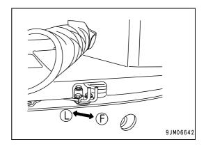
10. Pedal locking device (for the optional equipment control pedal)
