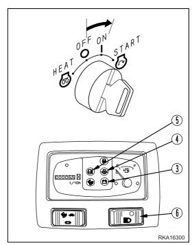
2) Press the light switch (6) and make sure that the work light functions correctly. If it does not function, this may be due to a faulty bulb, or to an interruption in the wirings, therefore it is advisable to contact a Komatsu Dealer, who will provide for the necessary repairs.
