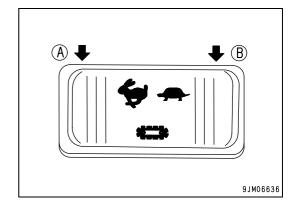
This is a two-position switch and is used to change over from high to low speed or vice versa.
