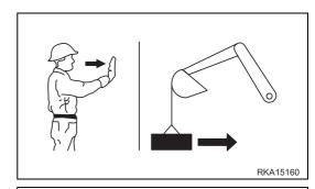
4 - BRING THE LOAD NEARER IN HORIZONTAL DIRECTION With an arm extended forwards and the hand in vertical position directed towards the signalman, move the hand in the direction of the movement to be carried out.
