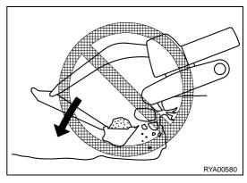
To make it easier to escape from the machine in case of emergency, set the tracks at right angles to the road shoulder or coast, with the sprocket at the rear, when carrying out digging operations.
