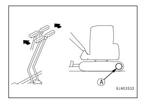
• When the sprocket (A) is at the front of the machine, pull the levers (3) slowly backward to move the machine off.
