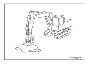
7. Lifting the machine by levering on the breaker bit with the bucket cylinder completely extended.
