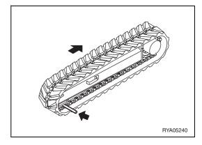
7. Make sure that the track tension is correct, that the track is correctly fitted in the sprocket and the idler roller, then rest the machine on the ground.
