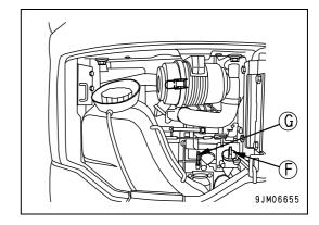
4. The oil level must be included between the H and L marks; if the level is near the L mark, top up through the filler neck (F), using oil suitable for the ambient temperature, as indicated in the lubricant chart
