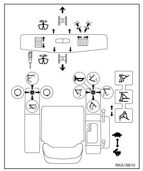
The control lever (2) is positioned on the operator's left and controls the arm and the turret swing.
