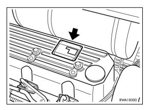
The exhaust gas emission plate is applied to the front side of the tappet cover.
