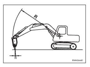
5 - Always check that the arm thrust is optimal, in order to avoid harmful and useless strokes.
