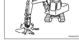
3 - Moving the tool while it is hitting the material to be broken.
