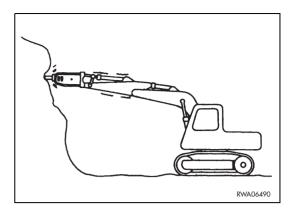
5 - Lever with the tool after thrusting it into the material to be broken.
