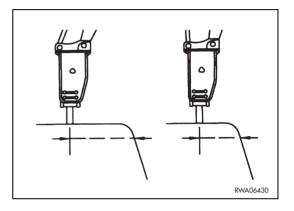
4 - To facilitate the sliding of the tool on its seat, check the thrust direction and always correct the hitting position of the hammer by means of the bucket and arm control.
