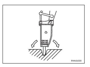
6 - Hitting the ground with the hammer bit.
