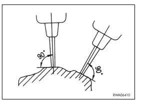
2 - Keep the pressure of the excavator on the hammer constant as the bit penetrates in the material.
