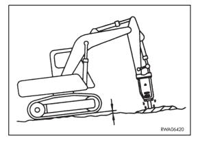
3 - When working on very hard materials, it is important not to keep hitting the same point for more than 30 seconds.Hit the same point for a few seconds and change position very frequently, in order to facilitate the breaking of the material.
