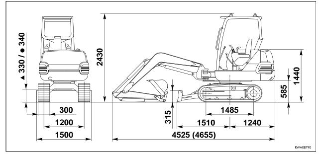
() Dimensions with long digging arm (L=1500 mm)
