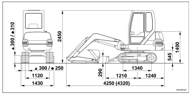
() Dimensions with long digging arm (L=1320 mm)
