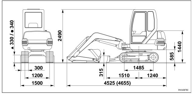
() Dimensions with long digging arm (L=1500 mm)
