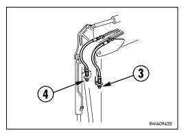
2 - If the pedal is pressed in (B) with the selection valve (1) control in (B), high-pressure oil is conveyed to the equipment through the right piping (4).
