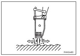
4 - Working with the hammer in horizontal position or even with greater inclination.
