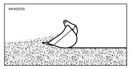
INCORRECT The bucket is pushed upwards and therefore is not filled completely.
