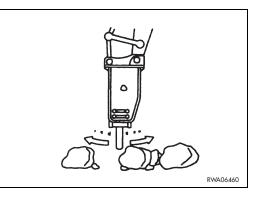
2 - Rotating the upper structure while using the hammer.
