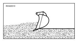
INCORRECT The bucket is thrusted downwards, slowing down the digging work.
