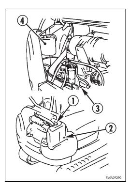
11 - Rotate the lateral counterweight to the closed position and close the engine hood.
