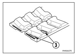
3 - When more than a half of the wires of the steel reinforcement positioned at the centre of the track are cut.
