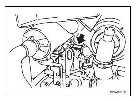
The exhaust gas emission plate is applied on the top of the engine cylinder head cover.
