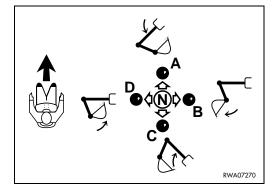
If the levers are operated in directions that are inclined with respect to the machine axis, simultaneous movements proportional to the angle of inclination are obtained, since the two hydraulic distributors corresponding to each single function are engaged at the same time.
