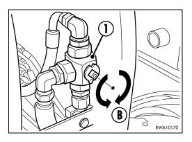
3 - If the circuit is arranged for the use of equipment with unidirectional flow (demolition hammer, etc.) and therefore with the selection valve (1) control in pos. (A), press the pedal (2) in (A) only, since the right piping (4) serves exclusively for the return of the oil to the tank.
