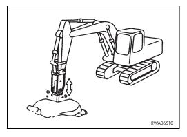
7 - Lifting the machine by levering on the hammer bit with the bucket cylinder extended to the end of its stroke.
