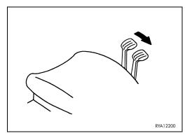
2 - Operate the levers (right and left) at the same time, shifting them forward to make the machine advance or backward to make it move in reverse.
