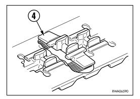
5 - If the rubber track tension is not sufficient after having been adjusted through the injection of grease, check the idler gaskets and if necessary change them or change the track.
