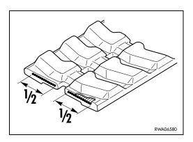
4 - When one or more steel reinforcement units (4) come off the track or are ejected due to the excessive tension.
