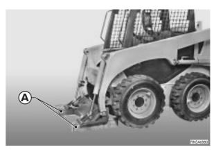
2 - Remove the pins (1) and retract the cylinder piston rods (2).
