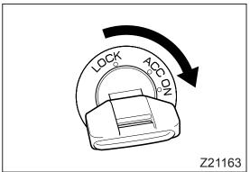
2. Turn the starter switch to the "ON" position.
