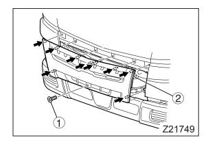
2. Remove the radiator grille by pulling outward on the clipped points in the order of the letters in the illustration.
