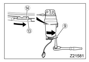
12. Install the fuel filter case by turning it clockwise. Turn the case until it stops. Make sure the proiection (3) on the case is in contact with the filter head 4.
