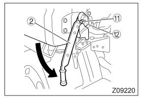
4. Push down lever B ② until the pin ⑪ engages with the latch ⑫.
