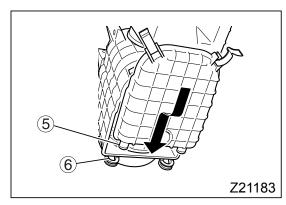
3. Install the cover on the case by inserting the projections ⑤ on the cover into the holes ⑥ in the case and then fasten the clamps.
