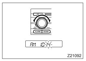
4. Adjust the minutes by turning the power/volume knob.
