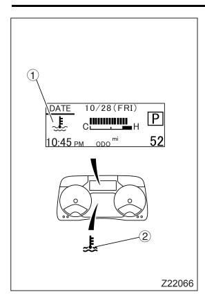
If the k warning lamp comes on, the multi-information display shows (red), and a buzzer sounds, the engine has overheated.
