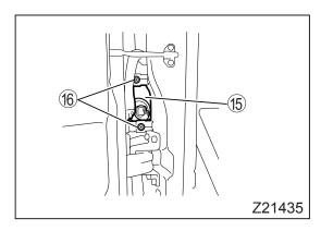
8. Open the door, then tighten the screws **behind** the front and side turn signal lamp **b**.
