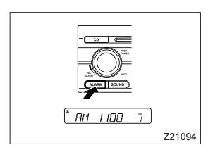
2. With the alarm time appearing on the display, give the "DISP" button a long press. A short beep will sound, and the hour part of the alarm time display will start flashing.
