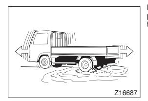
Move the gearshift lever between the "D" and "N" positions to rock the vehicle and thereby get it out of the mud, snow, or sand.
