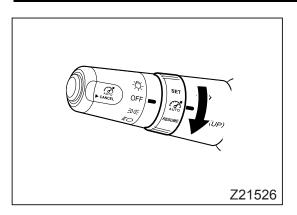
When the desired speed is reached, turn the SET/RESUME switch to the "SET" side for 1 second or longer. The vehicle will then cruise at the new, higher speed.
