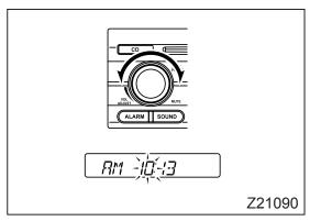
2. Adjust the hour by turning the power/volume knob.
