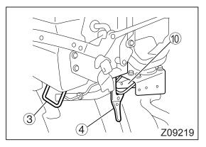
3. Still holding the tilt grip ③, lower the cab until the hook on lever C ④ engages with the cab mount ⑩.
