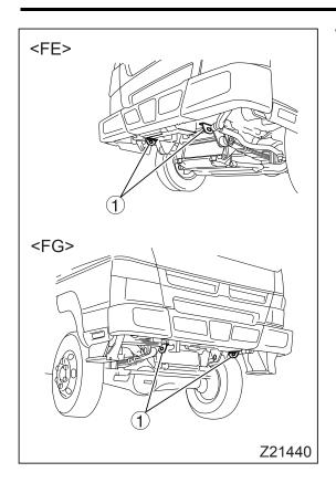
Never use the tie-down hook(s) ① under the frame for towing purpose. The tie-down hook is to secure the vehicle when transporting it. If the hook is used for towing, damage to the front bumper or frame may result.
