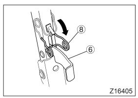
4. Still holding the tilt grip, insert the stopper ® into the notch of the lock lever.
