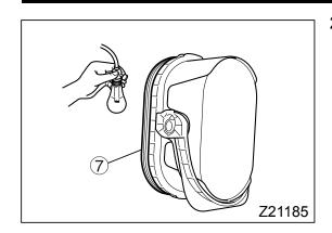
2. Put a light on the gasket side of the air cleaner element to check that there are no holes that allow light to leak in the element. Also check the gasket for cracks or other damage.
