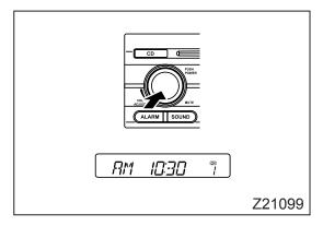
6. Press the power/volume knob to complete the alarm time setting.
