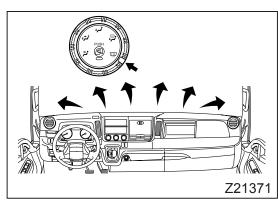
For airflow toward the windshield Place the mode selector dial in the position.
