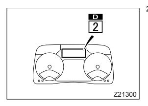
2. Check that the multi-information display is showing "D" and that the gear position indicator is showing "1" or "2".
