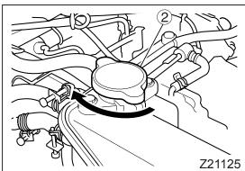
Check the coolant level. If the level is too low, add coolant.
