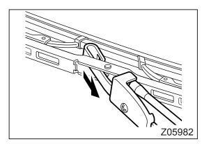
2. With the clip spring kept in the pushed position, press wiper ③ toward the wiper arm.
