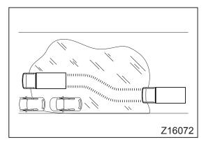
If a vehicle is driven on a slippery road or it is running with no or only light load, the wheels can lock and then skid when the brake pedal is strongly depressed. The ABS is a computer-controlled system that deters the wheels from locking by controlling the braking force on each wheel.
