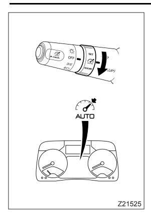
3. When the desired speed is reached, turn the RESUME/SET switch toward the "SET" side. The indicator lamp will illuminate indicating that the cruise control is activated. Now the desired speed is memorized, so release the accelerator pedal. The vehicle will run maintaining that speed automatically.
