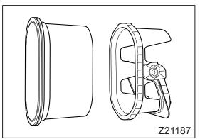
4. Replace the element with a new one if the check reveals a defective cleaner element or when the recommended replacement interval expires. Use a genuine cleaner element for replacement. Remove the air cleaner element from the case and replace it with a new one.
