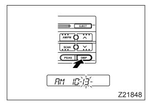
3. Press the "DISP" button. A short beep will sound, and the minute part of the time display will start flashing.
