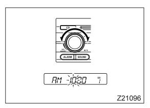
3. Adjust the hour by turning the power/volume knob.
