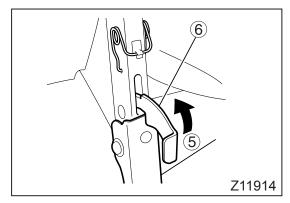
2. Hold the tilt grip to support the cab. Lift the lock lever (a) and fold the cab stay (a).
