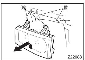
8. Raise the headlamp slightly to remove the tabs (5) from the holes (6), then pull it out toward you.
