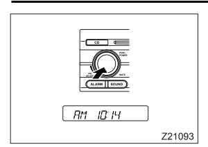
5. Press the power/volume knob to complete the clock setting.
