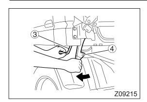
2. Grasp tilt grip ③ and pull lever C ④. The cab will rise slightly.
