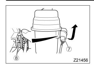
7. Disconnect the connector 7 from the fuel filter case. Do this by pulling the bottom part of the connector toward you to release the lock ® and then pulling the connector directly upward.
