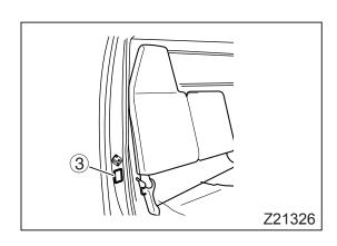
A label ③ indicating the vehicle information including the vehicle model, chassis number, and engine model is affixed to the pillar of the assistant driver's door.
