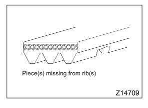
If a belt is cracked or otherwise damaged, have it replaced it as soon as possible. Belt replacement requires component disassembly. Please contact an authorized dealer to have the work done.
