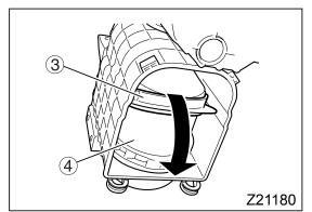
3. Pull element ④ straight down to remove.
