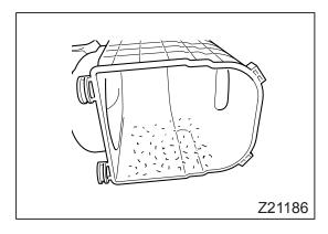
3. Clean the inside of the case and cover with a clean cloth. Clean the sealing sections with particular care.
