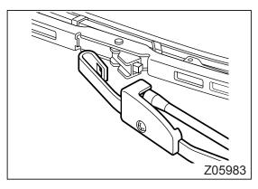
The wiper blade will come off the wiper arm. Install a new blade in the reverse order of removal.
