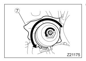
6. Remove the oil filter case by turning it counterclockwise. Use a rag ⑦ to prevent oil from dripping down.
