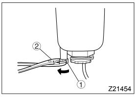
5. Loosen the drain plug ① by turning it in the direction of the arrow indicated in the figure to allow the fuel in the fuel filter to drain out. Use pliers ② or a similar tool to loosen the plug. After the fuel has been discharged, turn the plug in the opposite direction of the arrow.
