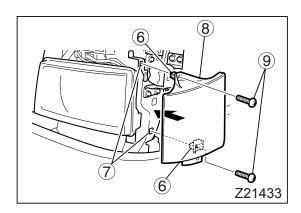
4. Insert the grommet ⑥ on the garnish ⑧ into the grommet hole ⑦, fit the garnish in place, and tighten the screws ⑨.
