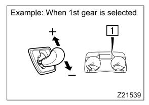
The "D" indication on the multi-information display disappears when the manual shift mode is engaged.
