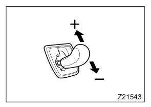
In the manual shift mode, the gear is fixed at the presently selected one even when the vehicle speed changes. So you should change the gear appropriately according to the vehicle speed.
