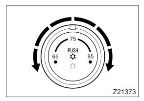
2. Set the desired temperature using the temperature adjustment dial.
