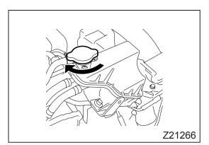
17. Screw the pressure cap down tightly by turning it clockwise.
