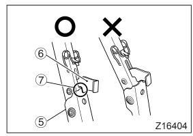
3. Hold the tilt grip and raise the cab until the end of cab stay ⑤ engages with the notch ⑦ of the lock lever ⑥. The cab is secured when they are engaged.
