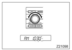
5. Adjust the minutes by turning the power/volume knob.
