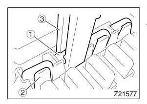
**1.4** How to remove the spare fuse Insert the puller ③ into the gap on the outer side of the fuse holder wall ② to remove the spare fuse ①.
