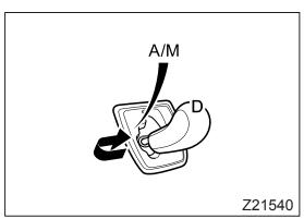
The gearshift mode also can be changed between "manual" and "automatic" each time you push the gearshift lever from the "D" position into the "A/M" position.
