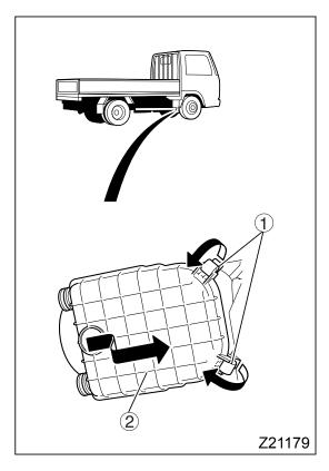
2. Move the lock lever 3 in the air cleaner element case to the "UNLOCK" position.
