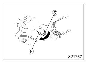
6. Open the radiator drain cock ⑤ to drain engine coolant.
