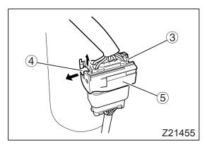
6. Disconnect the sensor connector ③. Do this after pulling up the connector's lock knob ④ and then pulling out the top part ⑤ of the connector.
