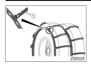
1. Place the chains over the tires with the hook ends of cross chains ① facing outward.
