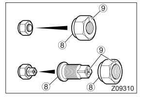
2. Mount the wheel so that the wheel bolts line up with the bolt holes in the disc wheel. Then, tighten the wheel nuts to hold the disc wheel in position. If the wheel nut has a spherical end 8, direct the spherical end toward the disc wheel.
