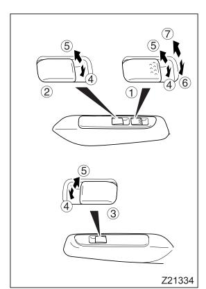
The power window switches function only when the starter switch is in the "ON" position.
