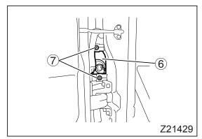
2. Open the door, then loosen the screws ⑦ behind the front and side turn signal lamp ⑥ until they spin freely.
