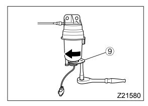
8. Remove the fuel filter case by turning it counterclockwise using the special tool 9 (separately available). Let the fuel inside the case drain out.
