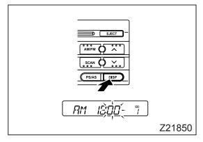
4. Press the "DISP" button. A short beep will sound, and the minute part of the time display will start flashing.
