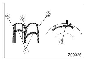
2. Connect the hook ③ of inside chain ②, leaving no excess links. Then, take up the slack in the inside chain by pulling cross chains ① for the inside tire outward.
