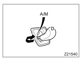
Push the gearshift lever into the "A/M" position if you want to change the gearshift mode from the manual shift mode to the automatic shift mode.
