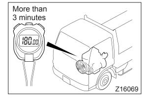
4. Turn the starter switch to the "ACC" position to stop the engine.
