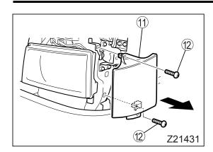
6. Remove the screws ② of the garnish ③, then remove the garnish toward the outside of the vehicle.
