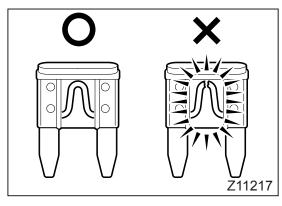
3. If a fuse is blown, be sure to select a spare fuse③ of the specified amperage for replacement.
