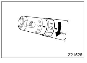
• To reactivate the cruise control while altering the set speed to a new speed, turn the SET/RESUME switch toward the "SET" side when the vehicle has reached the desired speed. The indicator lamp will light up, and the vehicle will continue running at the set speed.
