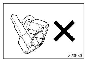
The handle of the engine immobilizer starter key is in contact with a metallic part of another key.
