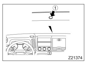
4. To stop operation, set the air volume adjustment dial to OFF.
