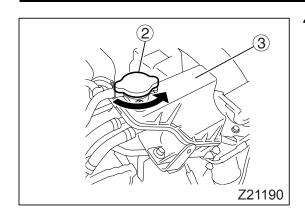
4. Remove the pressure cap ② of the surge tank ③ by turning it counterclockwise.
