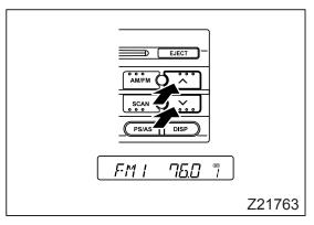
2. Make the frequency of your desired station appear on the display by using the "∧" or "∨" tuning button.
