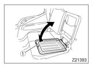
9 Center tray with magazine rack <option> Pull the lever ① on the center seat to fold the seatback. You will then be able to use the center tray and magazine rack.
