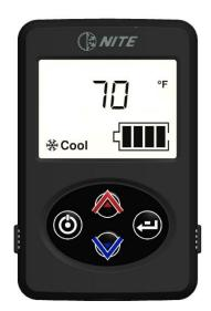
To view system runtime/hours – press ENTER until "Hrs" show on display. When hours are displayed, pressing ENTER for 7 seconds will reset the hours to zero.
