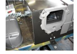
Attach Phoenix unit to floor of the truck using 1" X 5/16 hex head self-drilling screws.
