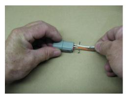
After wires are installed, slide the terminal lock into place, inside the connector
