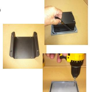
Before installing the bracket, secure the separator to the bracket with four 10 x 32 x 3/4" screws and lock washers provided.
