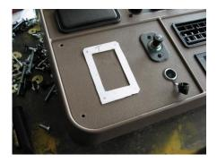
Drill starter holes for airsaw. Cut out marked section.
