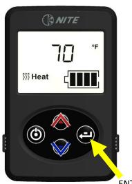
Changing BLOWER SPEED – press ENTER until display shows FAN and SPEED. Press up or down arrows to select 1-2-3 speed. After 5 seconds selection will be set.
