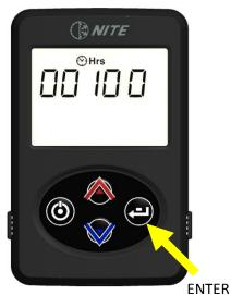
To change from °F to °C press ENTER until temperature symbol only shows – push the up or down arrow to change. After 5 seconds selection will be locked.
