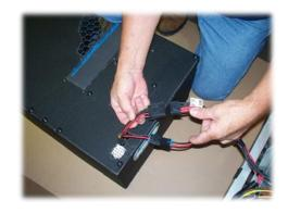
Secure harness at the unit to prevent stress on harness connectors.
