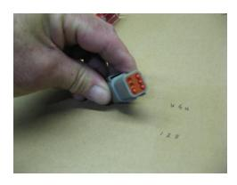
Install separator control wires into Deutsch connector
