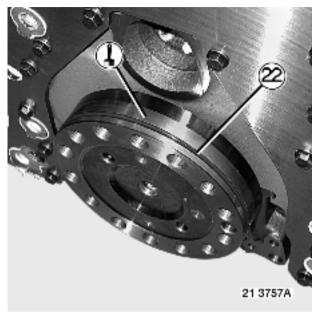
Lightly oil a new O-ring (22) and install. Fit pinion (21). Tighten bolts (20) to torque.
