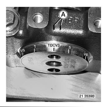
The camshaft top dead centre mark (TDC) must be positioned between the marks (A) on the camshaft front bearing cap.
