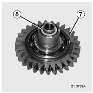
Replace O-ring **(8)** with a new O-ring. Depending on the assembly.
