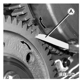
Slide a feeler gauge **(A)** with a thickness of **0.1 mm** between the teeth contact faces of pinions **(13 - 16)**. Preliminary tighten bolts **(10)** to a torque of **10 Nm**.
