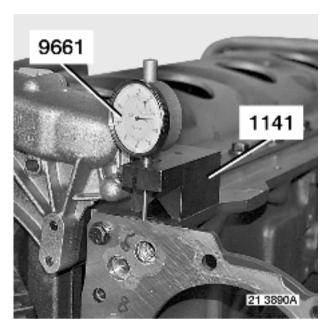
Check alignment of timing plate in relation to the bottom of the engine block. Correct distance  $0\pm0.25$  mm. Use tool 9661 + 1141.
