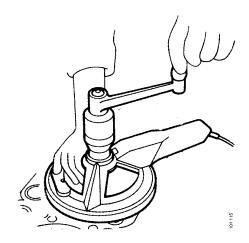
11. Move the bit back to the centre so that neither bit nor engine block is damaged when the tool is placed over the next liner seat.
