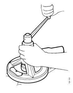
6. Lift the speed feed ring and withdraw the bit until the point is just inside the liner seat surface.
