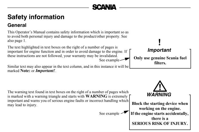
A list of the safety precautions to be followed when running and maintaining Scania engines can be found on the next three pages. Similar text can often be found at the relevant maintenance points, and here different levels of importance are attached to such text in accordance with the above description.
