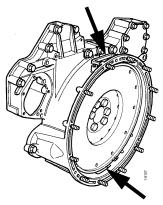
Openings for reading on the flywheel housing
