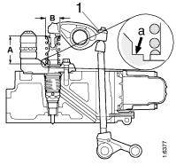
Measurement A= PDE31: 66.9 ±0.1 mm PDE32: 69.9 ±0.1 mm
