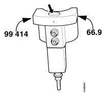
Piston above or below the flat surface. Adjustment necessary.
