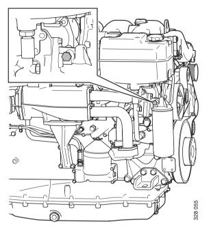
Connecting the oil pressure sensor, M16x1.5
