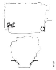
Examples of rigid engine suspension
