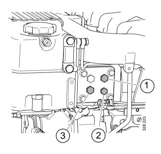
$Connection\ of\ sensor\ for\ coolant\ temperature\ and\ coolant\ pressure$
