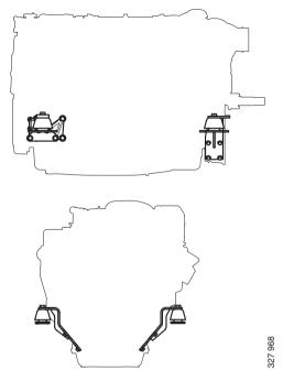
Examples of flexible engine suspension
