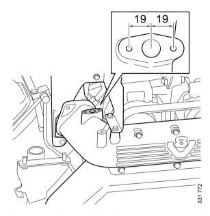
Connection of sensor for charge air pressure and charge air temperature,  $\emptyset$  16 mm, 2 x M6 screws
