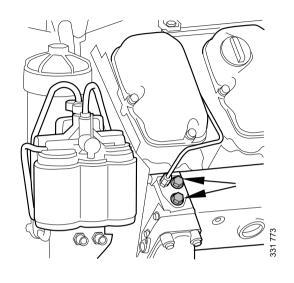
Connection of sensor for coolant temperature, G1/2". If necessary, an adapter can be ordered as extra equipment
