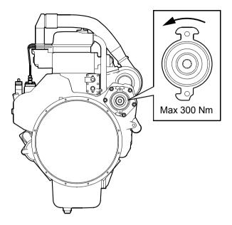
The power take-off is located low on the right of the rear of the engine, facing forward.
