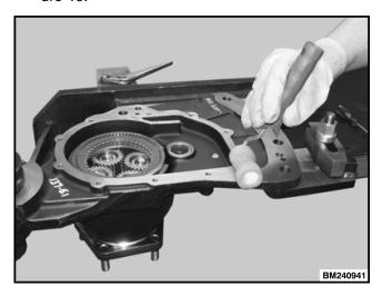
Figure 19. Applying Sealant to the Flange
