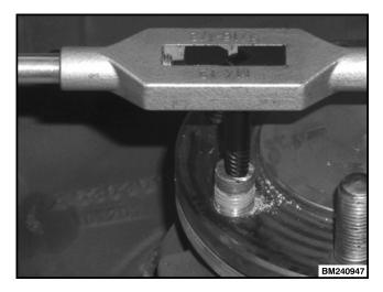
Figure 12. Removing the Stud
