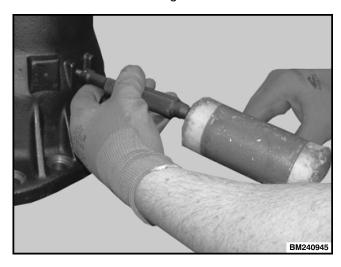
Figure 10. Installing the Breather
