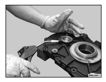
Figure 15. Removing the Cap
