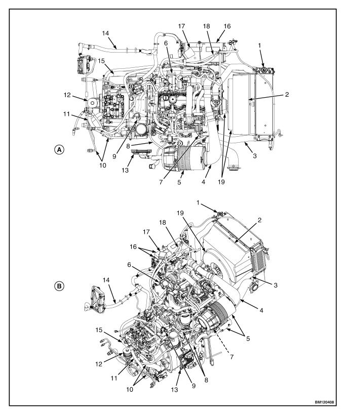
Figure 28. Kubota 3.8L Engine and Transmission for Lift Truck Models GLP/GDP40VX5/VX6; GLP/GDP45SVX5,GLP/GDP45VX6, GLP/GDP50-55VX (GP/GLP/GDP080, 090, 100, 110, 120VX) (H813) Manufactured Before February, 2012.
