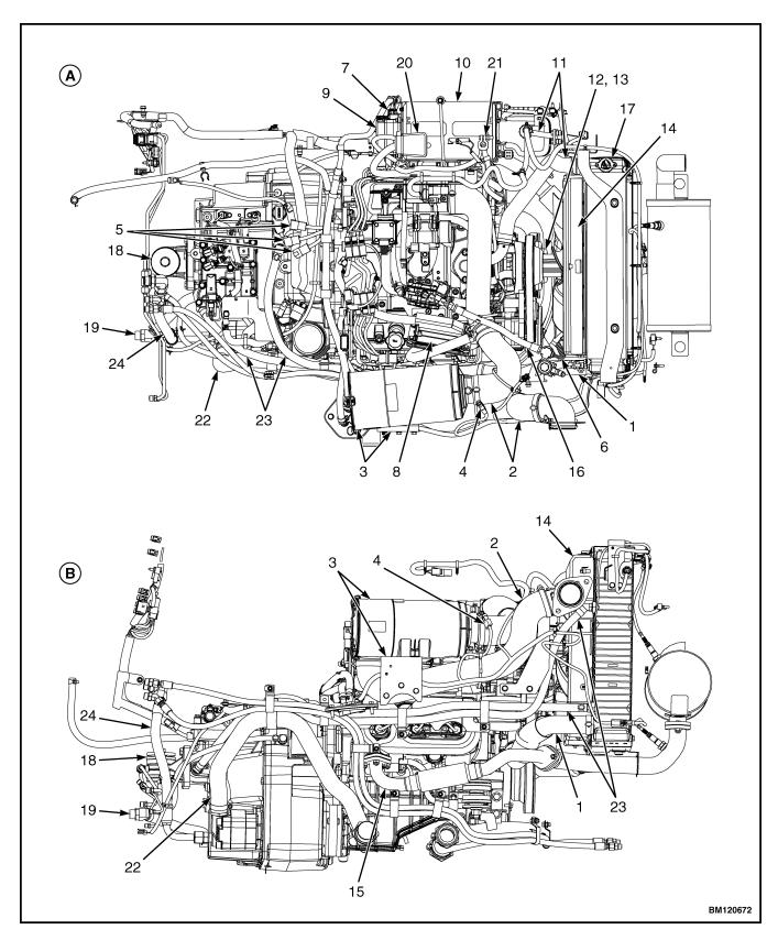
Figure 26. GM 4.3L LPG Engine and Transmission with Dual Hydraulic Tanks
