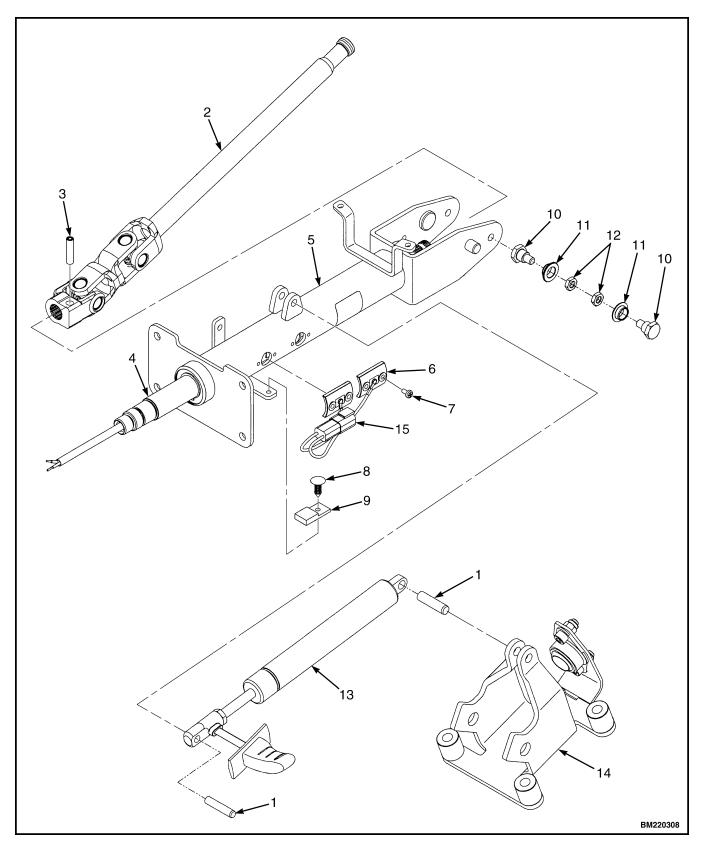
Figure 12. Steering Column Assembly, Lift Trucks Manufactured Before January, 2012
