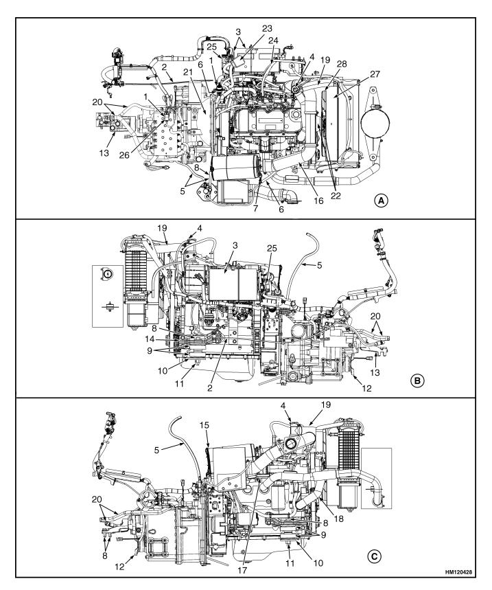
Figure 33. Cummins 4.5L Diesel Engine and Transmission
