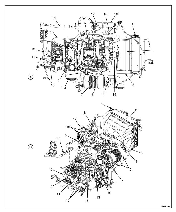
Figure 30. Kubota 3.8L Engine and Transmission for Lift Truck Models GLP/GDP40VX5/VX6; GLP/GDP45VX5, GLP/GDP45VX6; GLP/GDP50-55VX (GP/GLP/GDP080, 090, 100, 110, 120VX) (J813)
