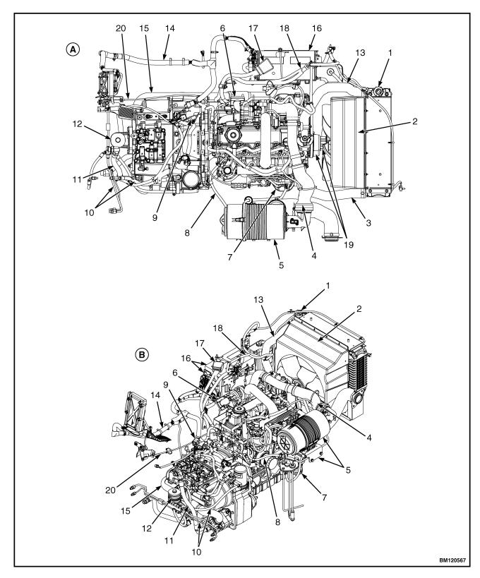
Figure 32. Kubota 3.6L Engine and Transmission for Lift Truck Models GLP/GDP40VX5/VX6; GLP/GDP45SVX5,GLP/GDP45VX6, GLP/GDP50-55VX (GP/GLP/GDP080, 090, 100, 110, 120VX) (H813)
