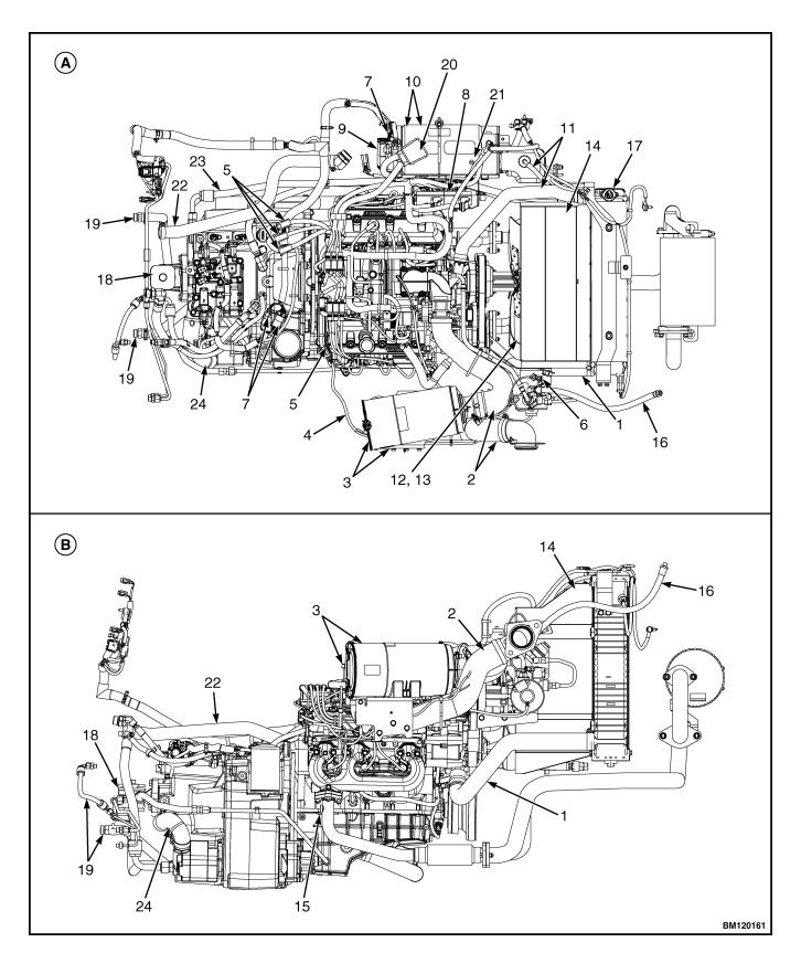
Figure 25. GM 4.3L LPG Engine and Transmission with Single Hydraulic Tank
