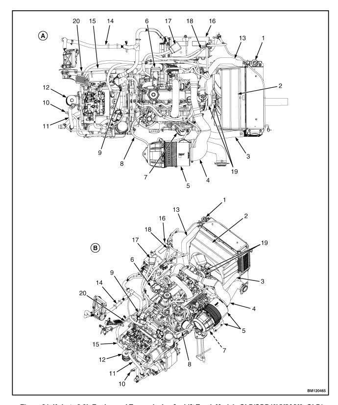
Figure 31. Kubota 3.6L Engine and Transmission for Lift Truck Models GLP/GDP40VX5/VX6; GLP/GDP45SVX5,GLP/GDP45VX6, GLP/GDP50-55VX (GP/GLP/GDP080, 090, 100, 110, 120VX) (H813)
