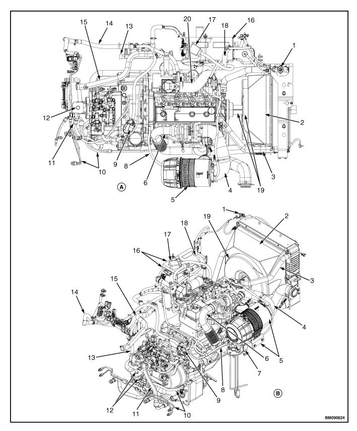
Figure 27. Cummins QSB 3.3L Diesel Engine and Transmission
