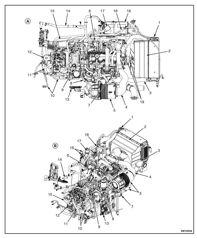
Figure 29. Kubota 3.8L Engine and Transmission for Lift Truck Models GLP/GDP40VX5/VX6; GLP/GDP45SVX5,GLP/GDP45VX6, GLP/GDP50-55VX (GP/GLP/GDP080, 090, 100, 110, 120VX) (H813) Manufactured After February, 2012.
