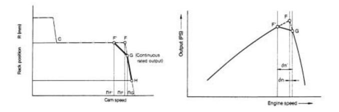
The torque spring thus provides for increasing of injection volume when speed decrease, to increase engine torque and in turn prevent engine stopping due to sudden increases in load, and also provide for strong engine output characteristics.
