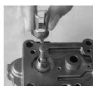
Remove the control sleeve.
