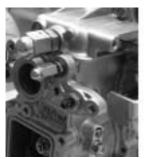
Set the engine speed at the no load max. speed. Pull the regulator lever and adjust the max. speed limit bolt to obtain the specified injection amount. Fasten the nut after completing the adjustment.
