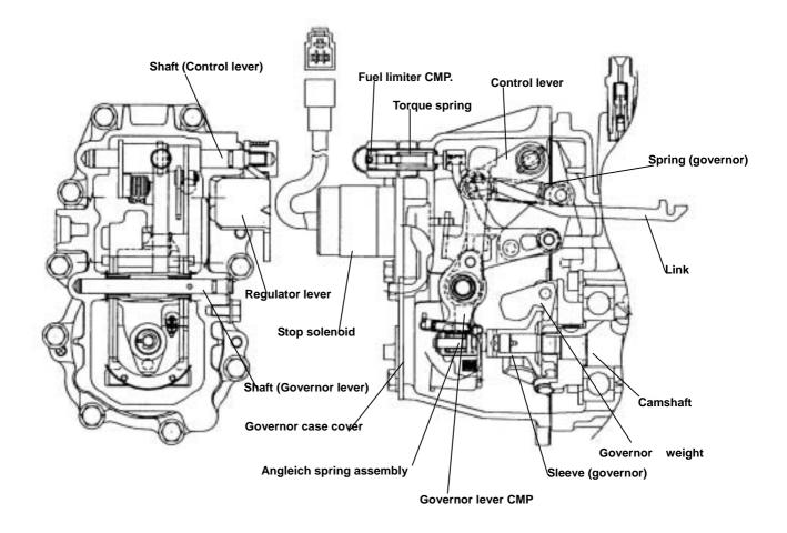
The governor weight mounted on the end of the fuel injection pump cam shaft rotates around the governor support pin, driven by the cam shaft, and is forced outwards by the centrifugal force acting on the weight.
