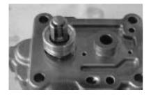
Install the control sleeve and spring retainer.
