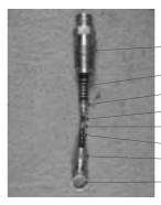
Holder(delivery Spring(delivery Valve(delivery Returnvalve (φ 2) Spring seat(return valve Returnspring Seat(delivery Packing(delivery
