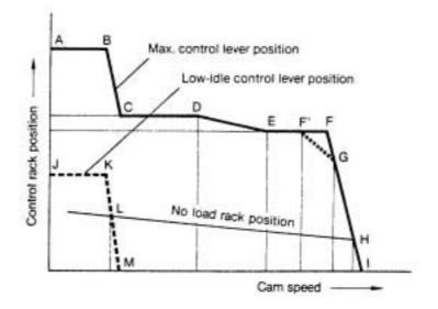
A-B : Fuel volume condition during starting. Volume is controlled by excess fuel spring.
