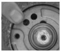
Align the camshaft's key groove with the embossed mark on the body.
