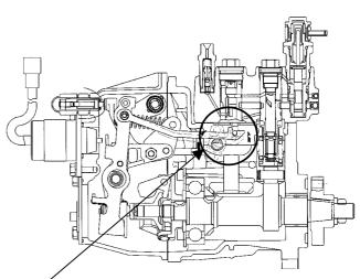
Rotating the link lifter will move the inside link upward/downward, so the control rack may be engaged/disengaged.
