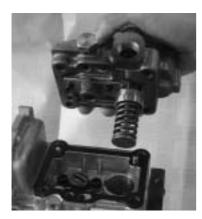
Remove the hydraulic head CMP.
