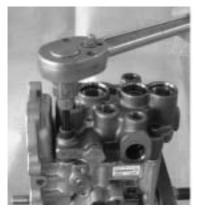
Remove the hydraulic head CMP fixing bolt.
