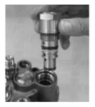
Install the holder with new O-ring, (timer).
