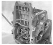
Remove the retainer, (bearing) fastening bolt.
