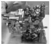
Pull the governor assembly slightly to check that the link is engaging securely.
