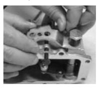
Pierce the spring, (control lever) through the lock nut, (control lever) and fasten it to the thread of the shaft, (control lever).
