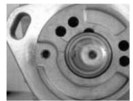
Position the camshatt key groove as shown in the illustration.
