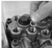
Install the new packing, (delivery valve seat).
