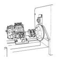
(4) Remove the plug in the oil fill hole on the top of the governor case, and fill the pump with about 200cc of pump oil or engine oil.
