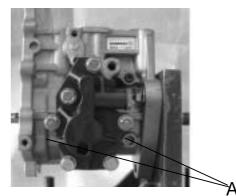
Remove the feed pump. Do not loosen two bolts (A)
