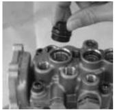
Install the plug, (distribution shaft).
