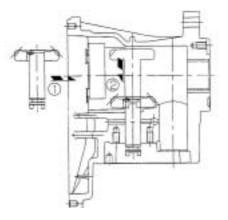
Attaching transmission shaft CMP
