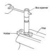
NOTE: Use a special box spanner for the hole type (the thickness of the two nozzle nuts is 15mm(0.5906in.)).
