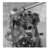
Install the hydraulic head CMP fastening bolt.
