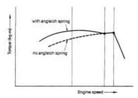
(6) Necessity of torque spring and function
